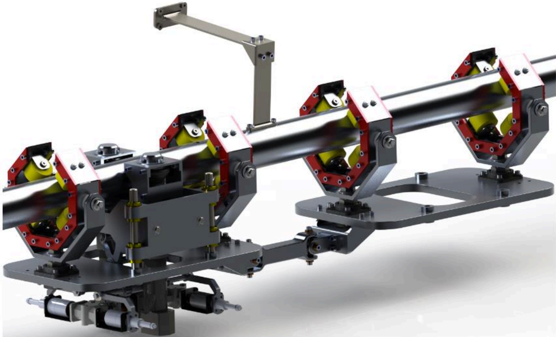
Figure 12: The DORIS mechanical design, showing a straight section of the rail with a support, the traction module, the passive module and a double Cardan joint used to couple the two modules. (Carvalho et al., 2013)
