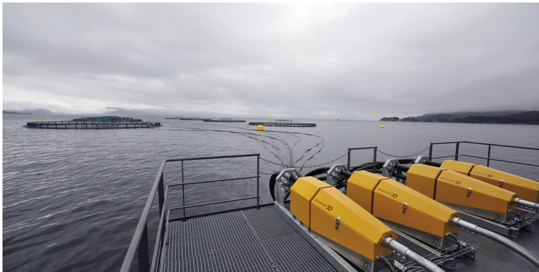
Figure 2.4: Central feeding system, Akvasmart (AKVA Group ASA, 2015b)
