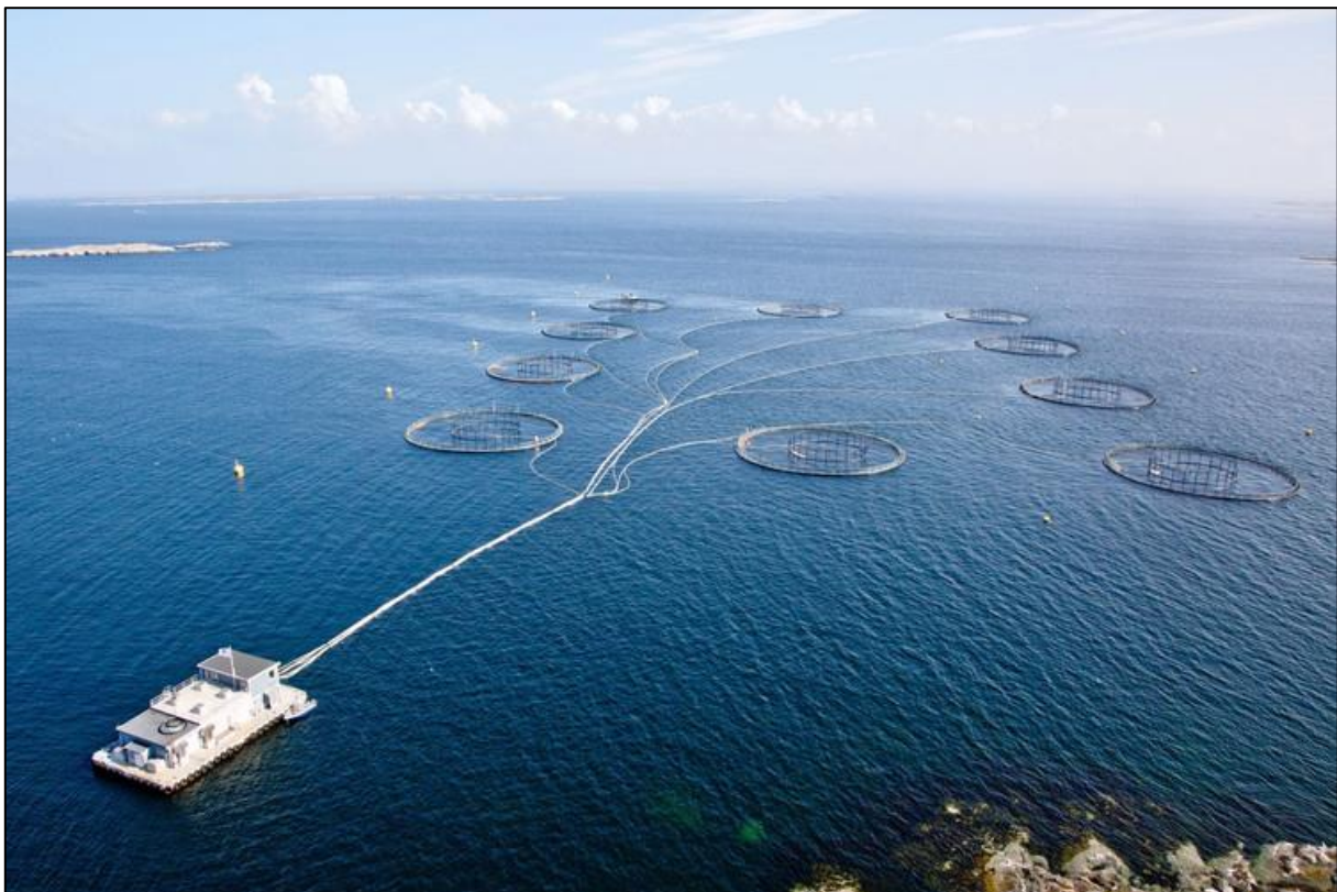
Figure 3. A barge monitors and pumps feed to salmon in net pens at Marine Harvest farm in Norway [17]
