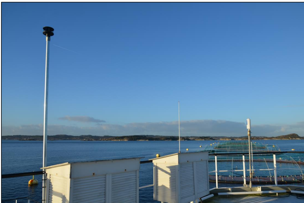
Figure 25. Wind measurement system. The wind sensor is a WindSonic ultrasonic wind sensor.
