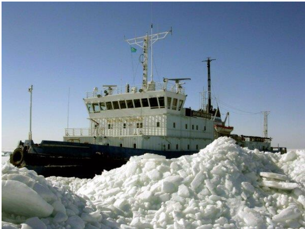
Figure 2.8 – Breaking Supply Vessel carrying goods in severe ice conditions of the Northern Caspian Sea, Kashagan field.
