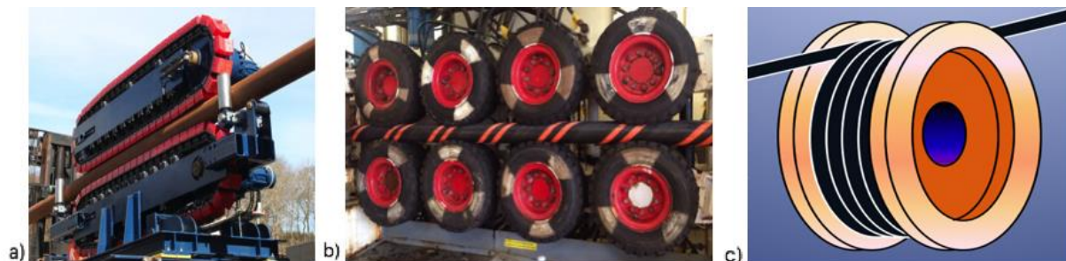
Figure 19: Cable tensioners; a) Caterpillar (4 All Ports), b) Linear Engine (Photo: Louise Våbenø), c) Capstan (Solberg, 2016).
