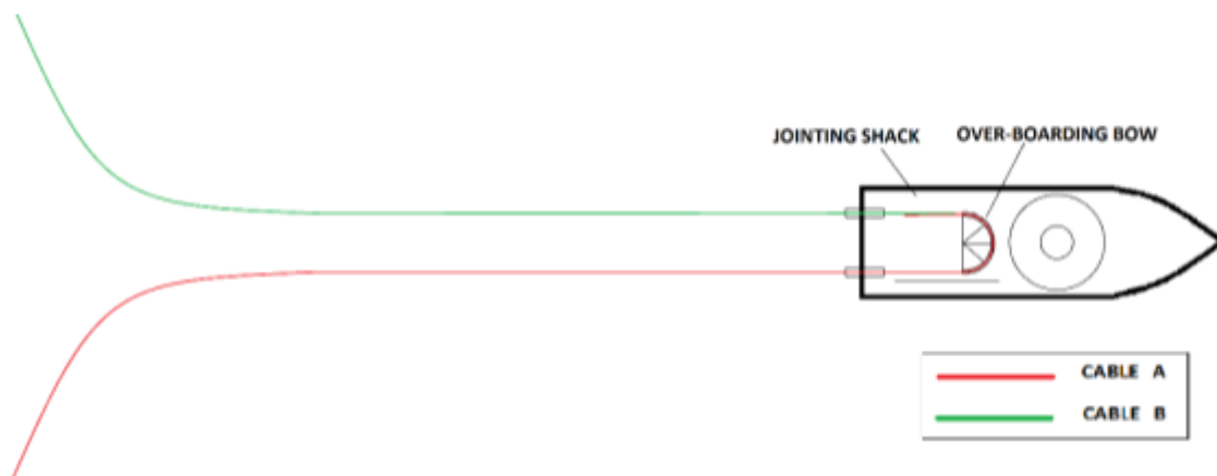
Figure 27: Hair-pin joint of two cables.
