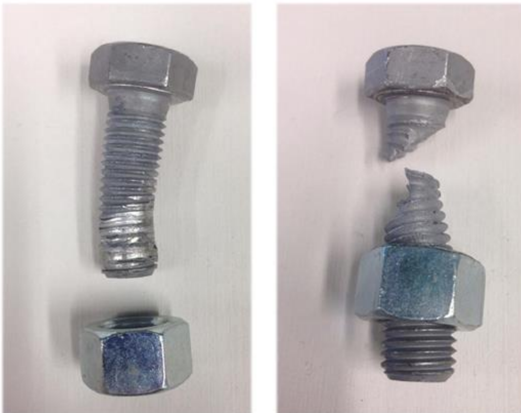
Figure 5.12: Failure at nut (left) and failure at bolt (right)
