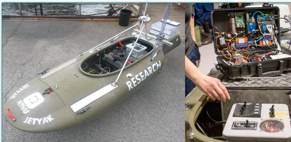
Figure 4.7. USV Jetyak - platform and interior
