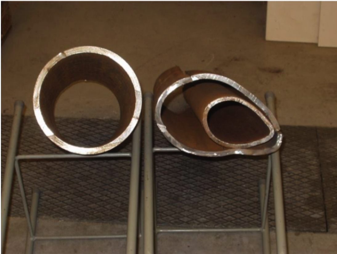
Figure 6: Collapsed production- casing and tubing [11]
