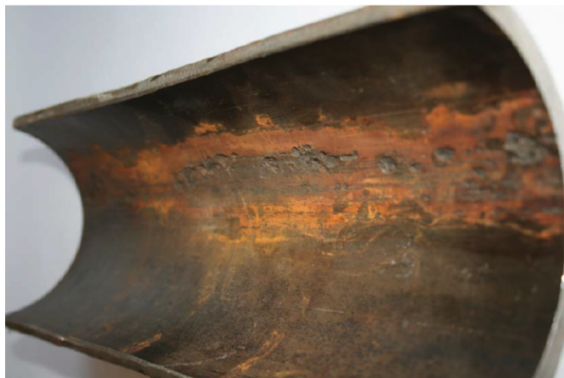
Figure 10: Locally corroded L80 13Cr tubing [5]
