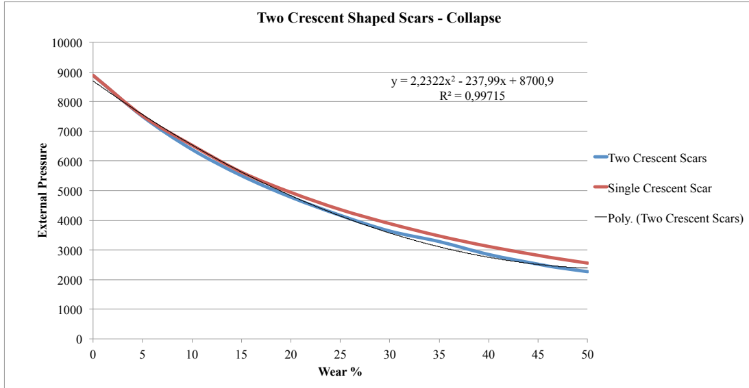
Figure 81: Safe and failure zone for operating external pressure
