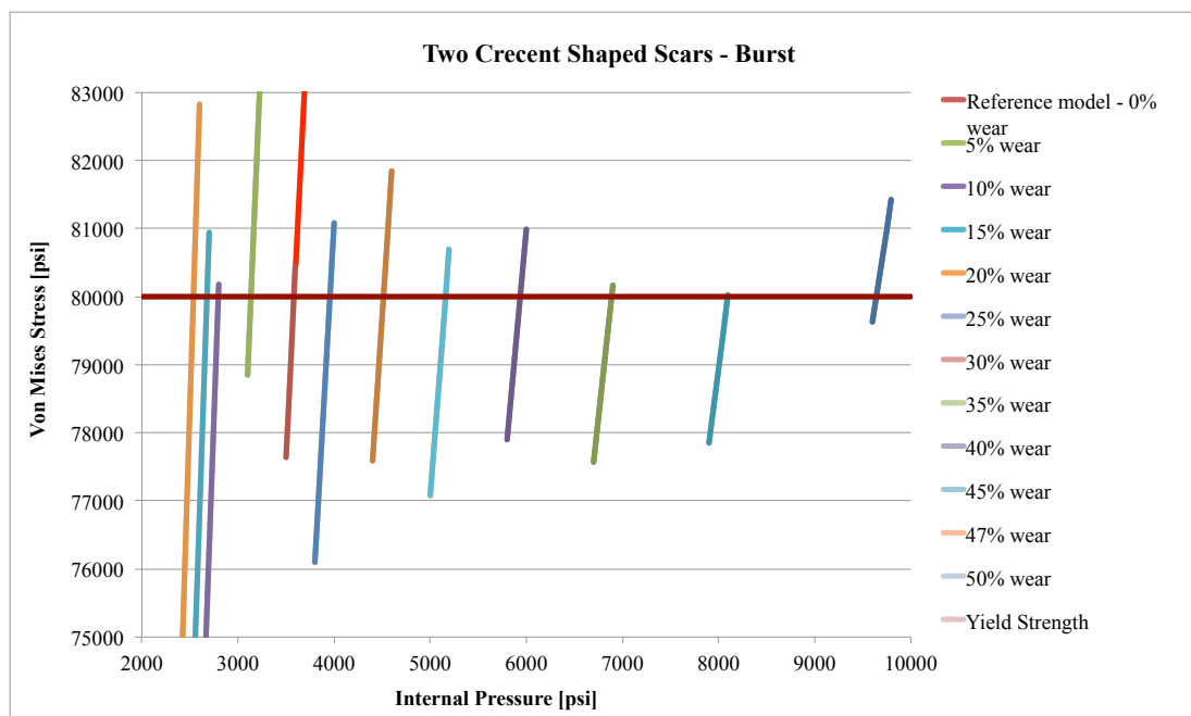
Figure 67: Internal pressure and the respective Von Mises Stress for different wear depths
