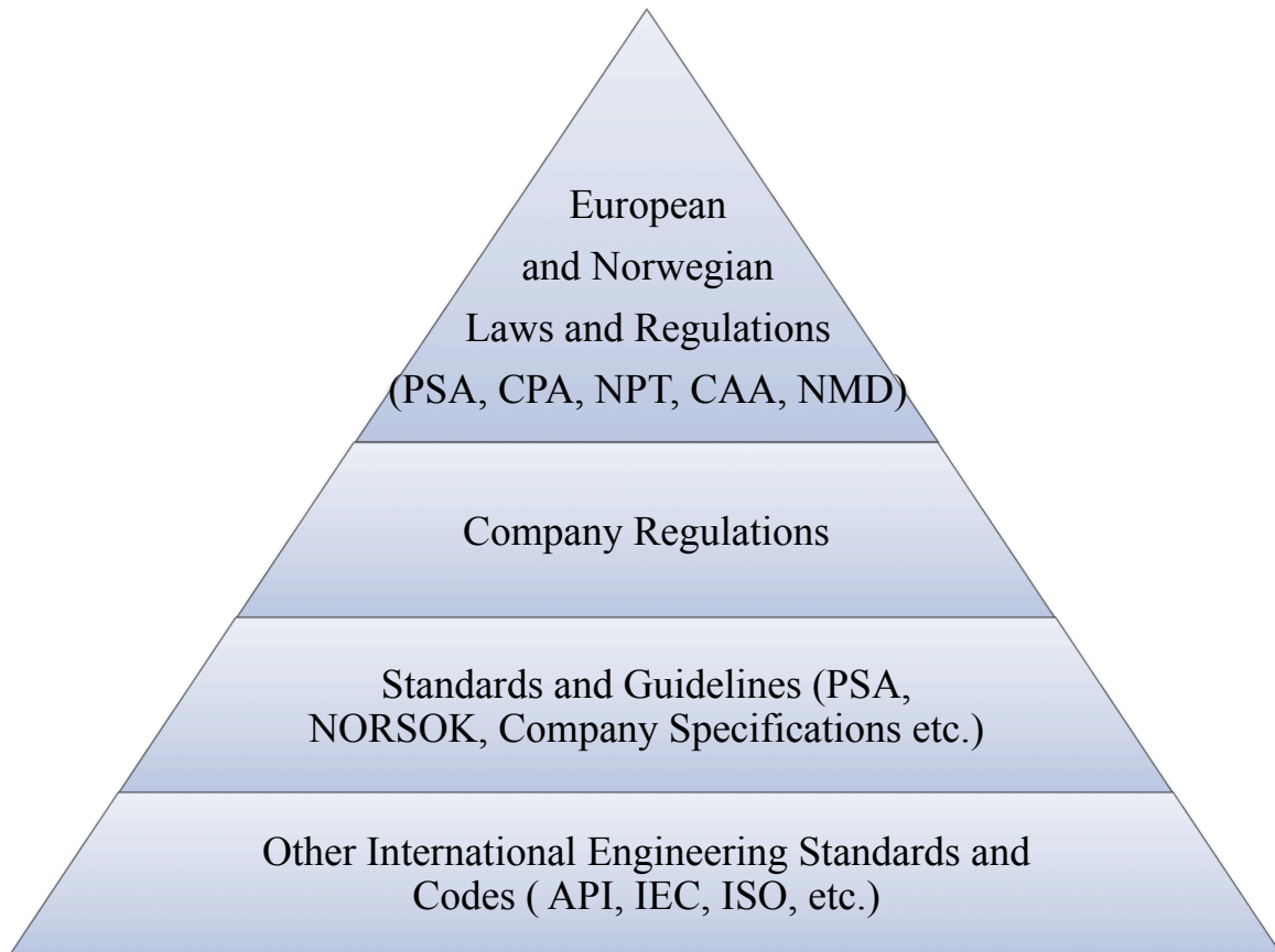
Figure 2.1: Hierarchy of Regulating Bodies on the NCS. PSA: Petroleum Safety Agency, CPA: Climate and Pollution Control Agency, NPT: Norwegian Post and Telecommunication Authority, CAA: Civil Aviation Authority, NMD: Norwegian Maritime Directorate.
