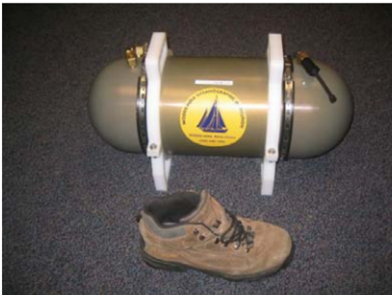
Figure 5.15: The TETHYS Mass Spectrometer 46 . The compact sensor is almost as small as a shoe.
