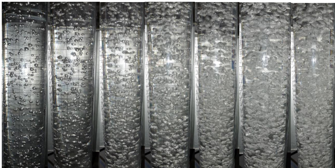
Figure 22 Flow pattern between the two pressure taps at 0.2; 0.5; 1.0; 1.5; 2.0; 2.5; 3.0 SPLM of gas (air) for the gas sparger with sintered filter cartridge injector
