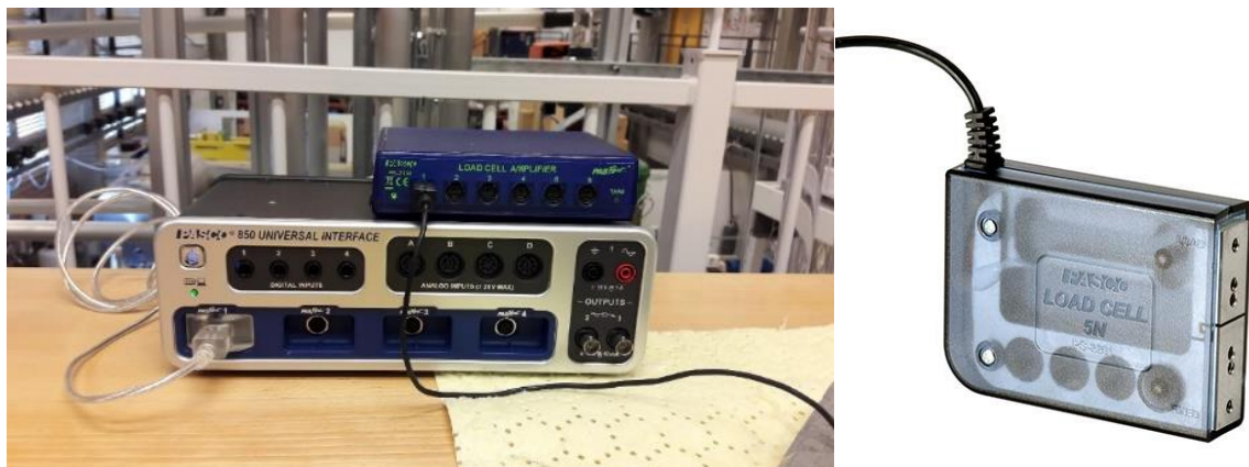
Figure 38 a PASCO 850 universal interface, 6-pin mini-DIN connector and PASCO 5N Load Cell PS-2201
