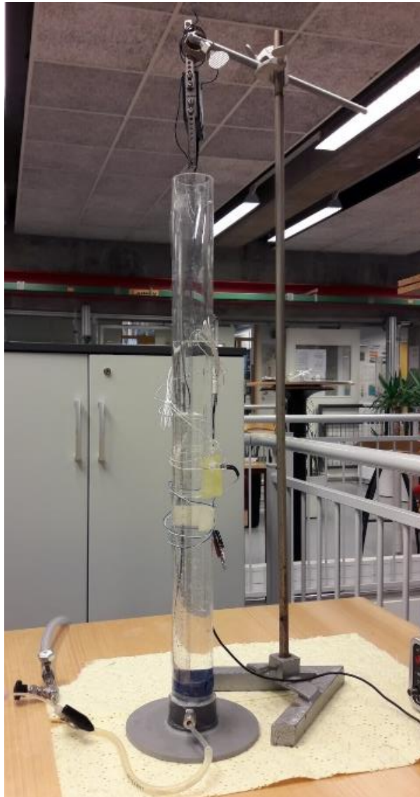
Figure 41 The Feasibility setup with the PASCO 5N Load Cell PS-2201
