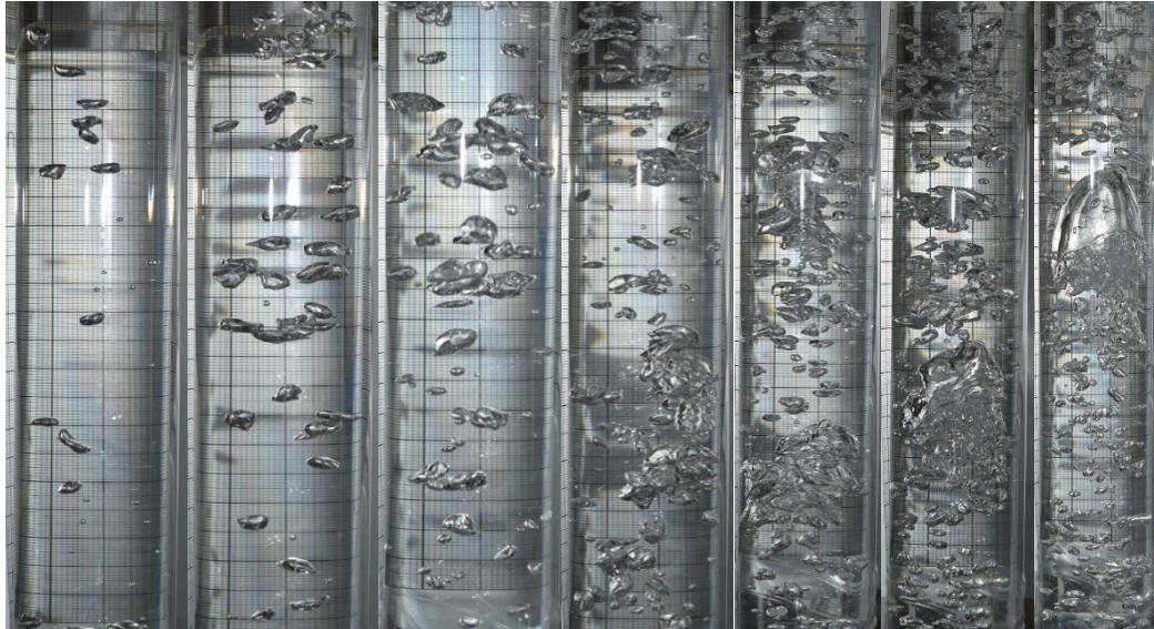
Figure 21- Flow pattern between the two pressure taps at 0.2; 0.5; 1.0; 1.5; 2.0; 2.5; 3.0 SPLM of gas (air) for the swagelok nipple 1/16 inch injector [8]
