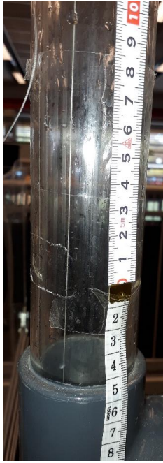
Figure 42 Sowing thread sticking to the pipe
