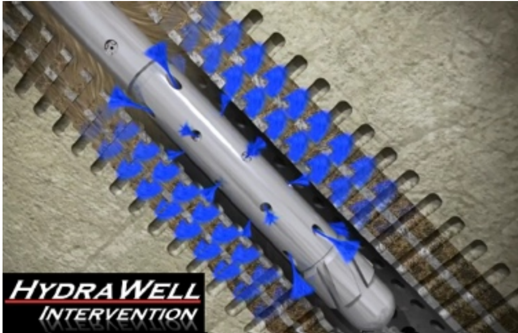
Figure 7 - Illustration of the washing process performed with HydraHemera [12]
