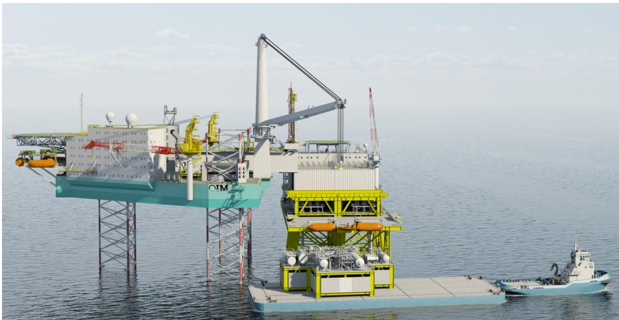
Figure 9 - DWP Self-Elevating Plug & Abandonment and Heavy Lift Crane Jack-Up Unit
