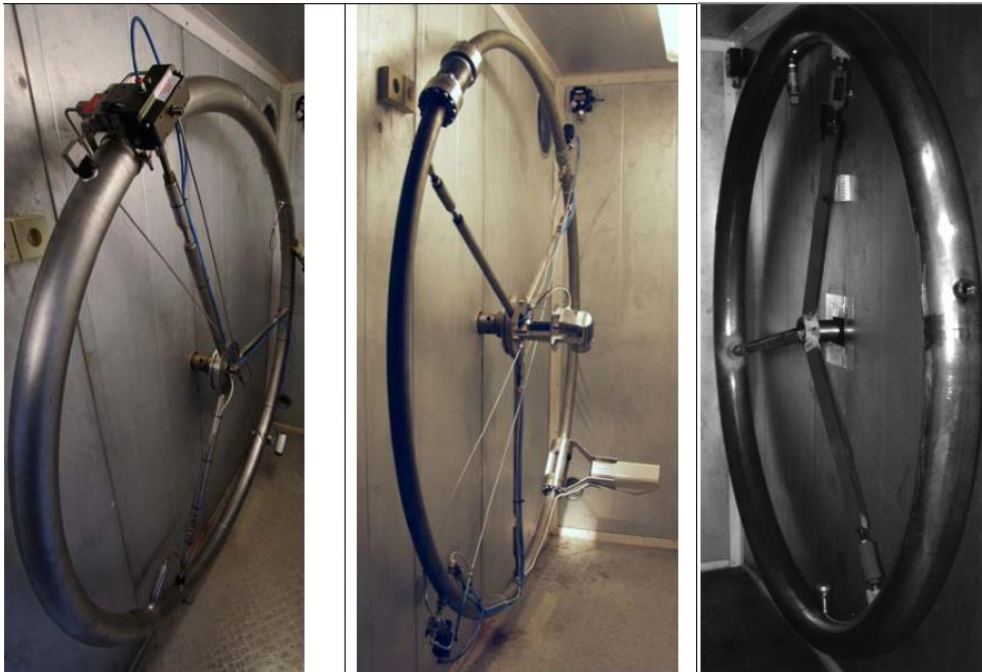
Figure 5.2: SINTEF wheel flow simulators [29].
