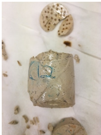
Figure 4.8 Core K12 after creep failure
