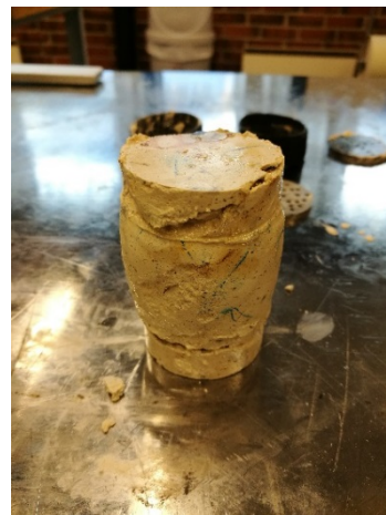
Figure 4.9 Core K5 after creep failure
