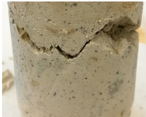
Figure 4.18 Core K6 after failure
