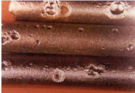
Figure 25 Hydrogen sulfide corrosion [26]
