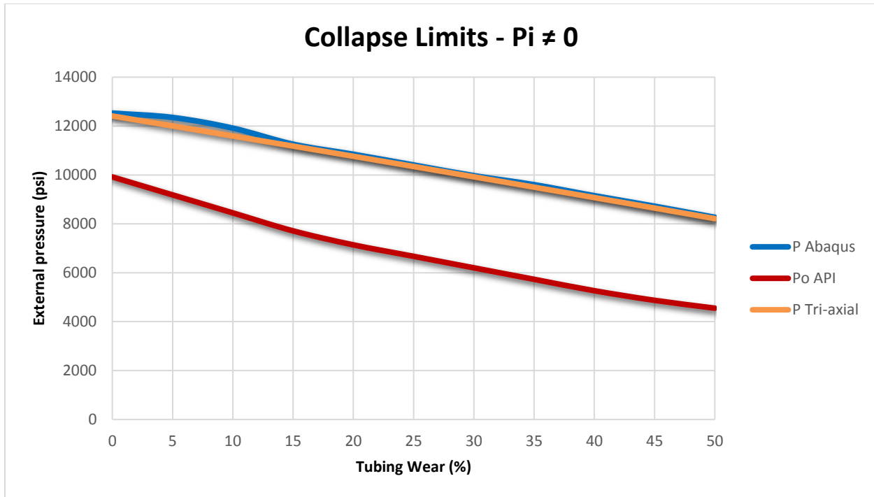
Figure 76: Simulation vs. theoretical results for P_i \neq 0 - collapse case
