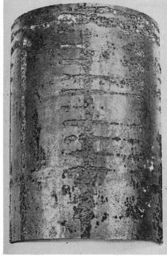
Figure 28 Bacterial corrosion outside of casing [31]
