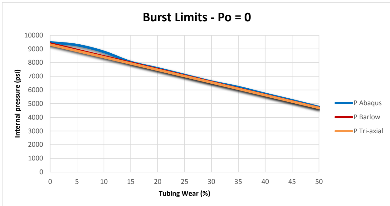
Figure 72: Simulation vs. theoretical results for P_o = 0 – burst case
