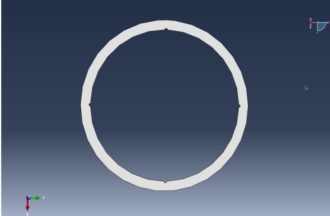
Figure 79: Tubing geometry for four points of local damage due to pitting corrosion
