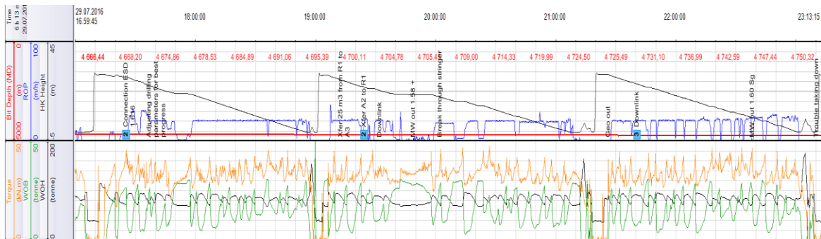
Figure 108: The varying torque and weight seen when starting drilling on the second run [6]
