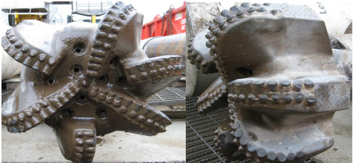
Figure 65: Bit condition after POOH
