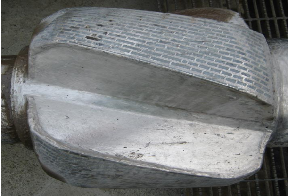
Figure 66: Stabilizer condition after POOH
