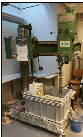
Figure 12: Coring Machine to drill out the outcrop Kansas Chalk.
