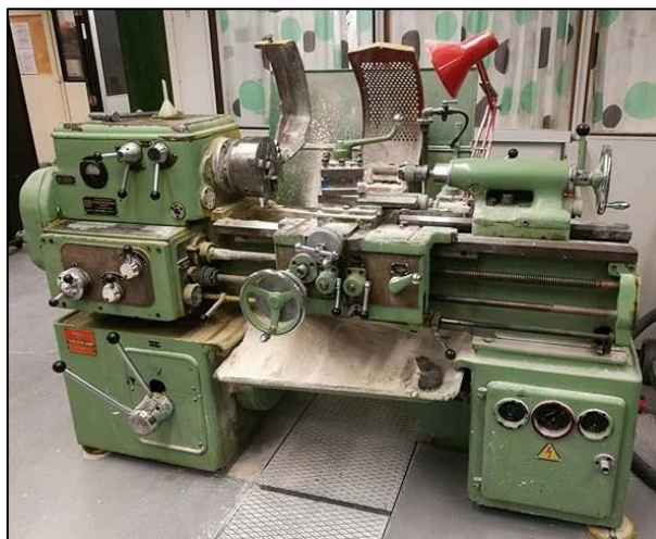
Figure 13: Lathe machine used to shape the oversized cores.
