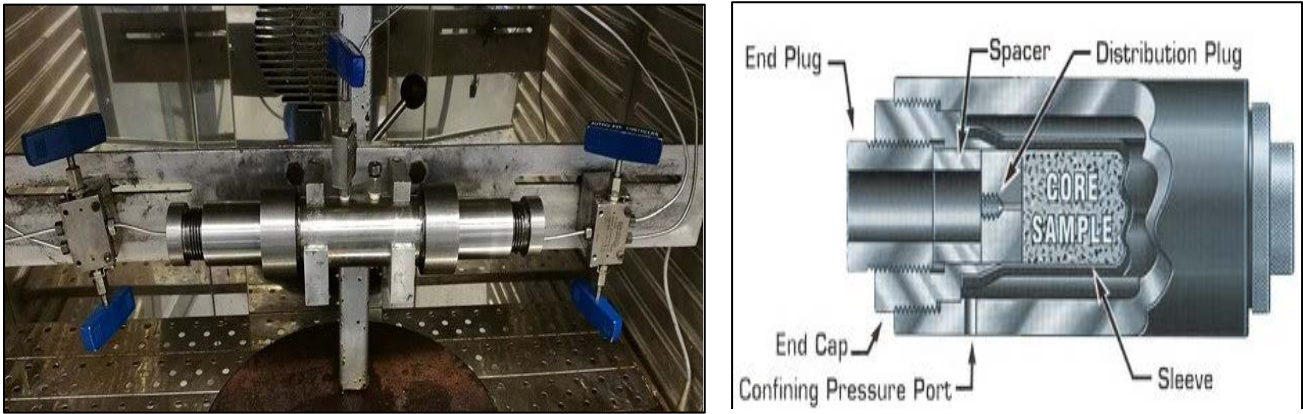
Figure 21: Left: Actual Hassler type core holder at the lab. Right: Sketch of Hassler type core holder.
