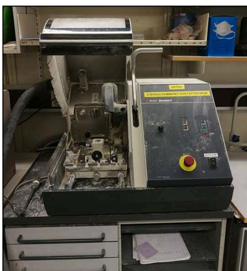
Figure 14: Diamond cut-off used to cut the cores to the required length.
