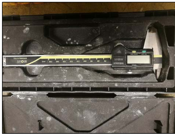
Figure 15: Calliper used to measure the length and diameter of the final cores.
