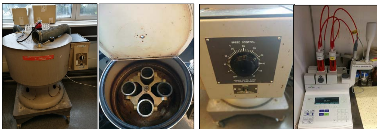
Figure 9: From left to right: 1) Centrifuge. 2) Inside of the centrifuge. 3) Centrifuge's Speeds. 4) Titration equipment.
