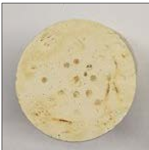
Figure 64: Core K4 Inlet removed from the rest of the core for density and specific surface area analysis.
