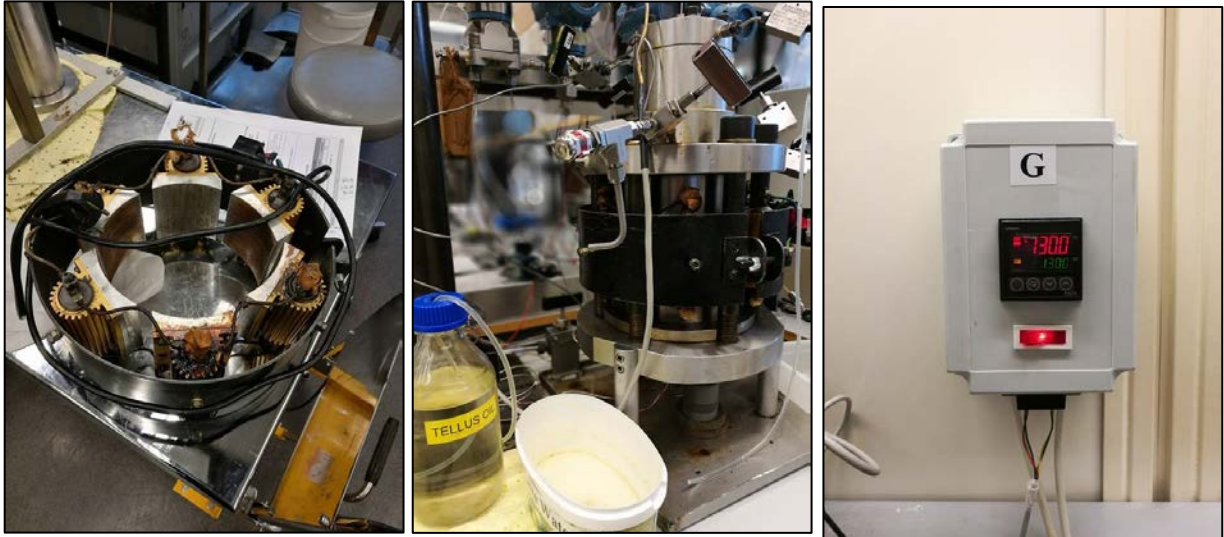
Figure 24: Left: Heating Jacket. Middle: Heating jacket attached to the confining chamber in a triaxial cell. Right: Omron Control Box keeping the temperature constant at 130°C.
