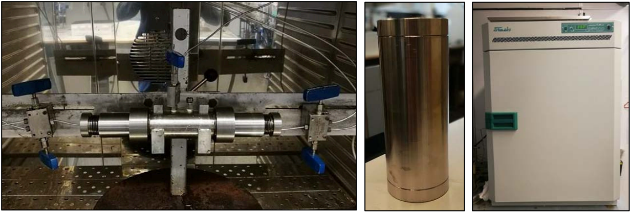
Figure 20: Left: Hassler's Cell Core Flooding Setup. Middle: Aging Cell. Right: Oven used for aging.
