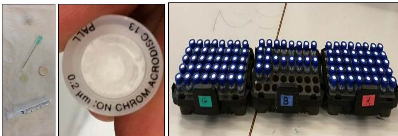
Figure 37: Left: Elements used to prepare the sample for the IC. Middle: Syringe chromatographer filter. Right: IC samples prepared.
