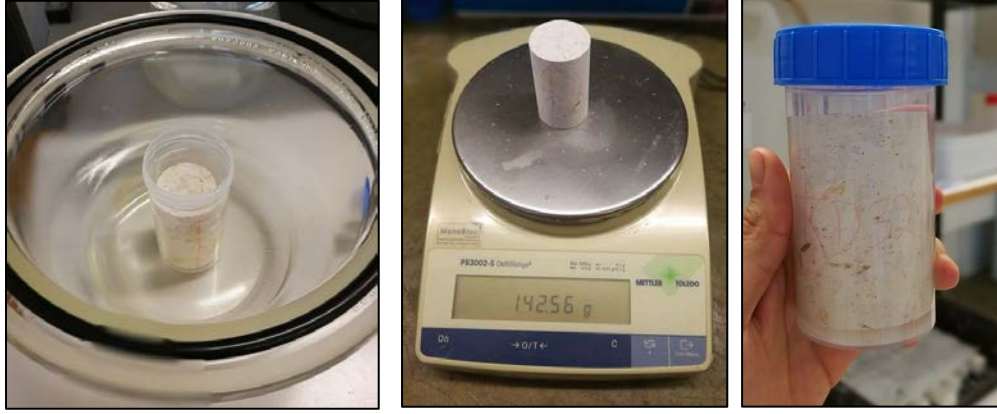
Figure 18: Left: Saturated core. Middle: Weight of the saturated core. Right: Saturated core placed inside of cylindrical container.
