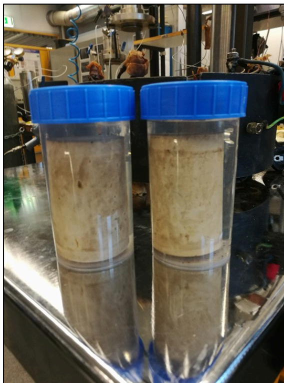
Figure 62: Mixed wet cores K7 and K8 preserved in distilled water after being removed from the triaxial cell.
