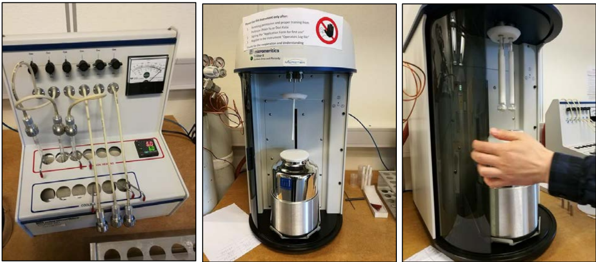
Figure 42: Left: Degasser set at 60°C containing the three sample tubes. Middle: Instrument with the liquid N 2 container in the bottom. Right: Samples attached to the instrument.
