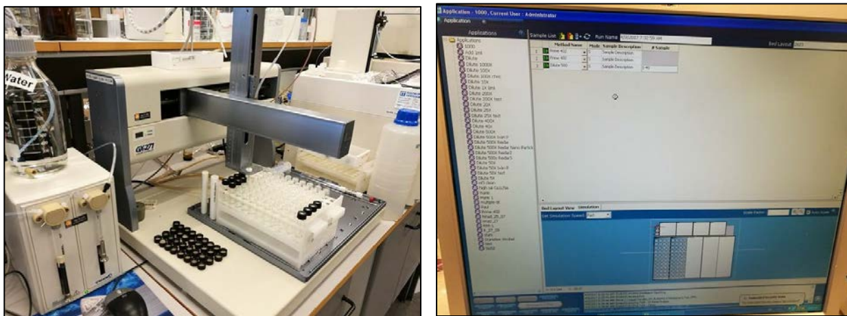
Figure 36: Left: Liquid handler diluting the sample. Right: Trilution software showing the program used for dilution: The lines were cleaned twice and the samples were diluted 500 times.
