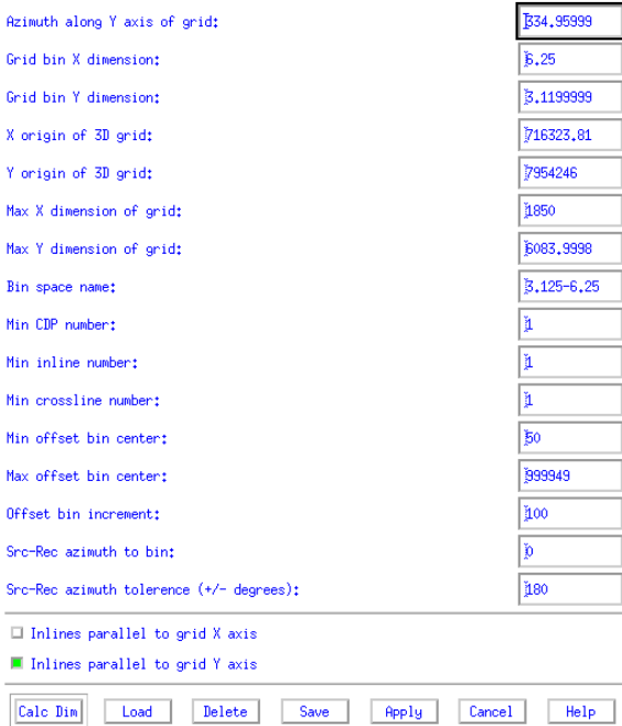
Figure 6 – Definition of bin size and numbers of dx and dy cells. This example show grid bin x equal to 6.25 and for y 3.125 m.
