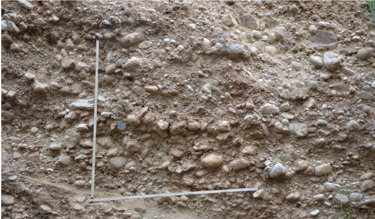
Figure 15: Example of how the average clast size of an outcrop is measured. The ten largest conglomerate clasts within an area of 1x1 m is measured and averaged according to Tucker (2011).
