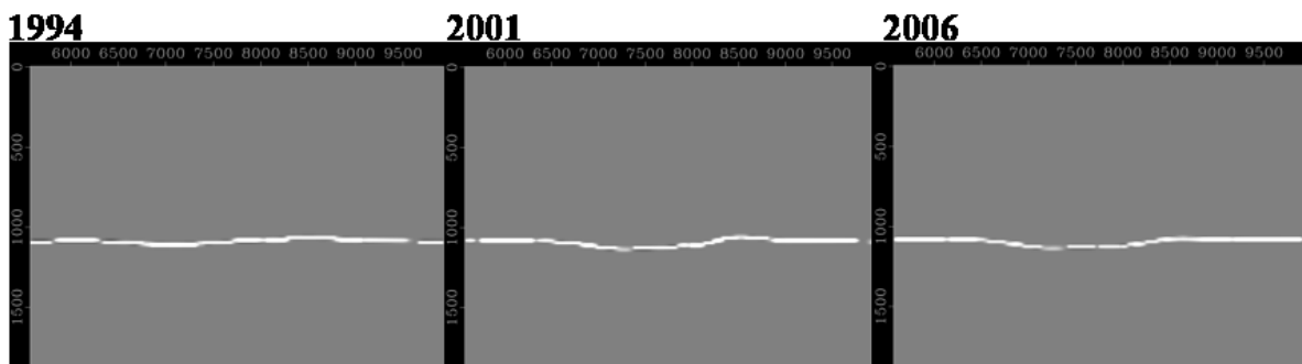
Fig. 4.7: Unmigrated interpretation of base horizons in each dataset. The velocity model developed with the WEMVA method aims to relocate horizons of the monitoring datasets to match the depth of the baseline survey of 1994.
