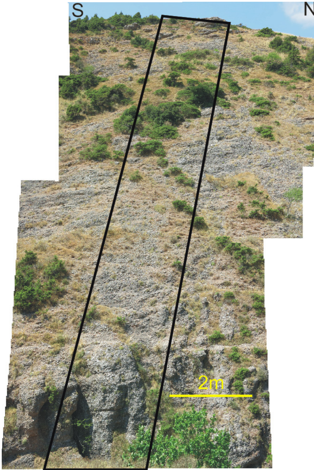
Figure 49: Composite photo of Section 2 – East from bottom to top. Notice the degree of erosion compared to Section 1, and the lack of thick and pronounced conglomeratic beds anywhere but at the base. The location of this photo is shown in Figure 45.
