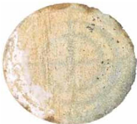
Fig. 6. A picture showing filter cake (white substance) formed at the core inlet during injection of 0.5 wt.% colloidal solution containing 0.08  $\mu\text{m}$  size particles into Kirby sandstone core. The narrow pore channels in Kirby core prevented some of the particles from penetrating the inlet of the core.
