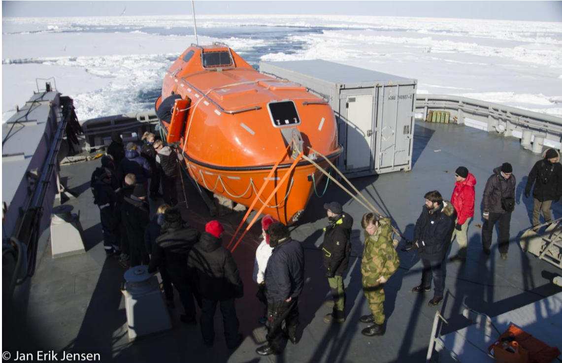
Boarding of lifeboat for O 2 /CO 2 tests.
