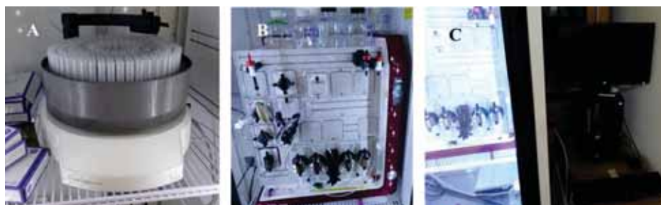
Figure 3.31 – Ion-exchange chromatography equipment Äkta™ Pure from GE Healthcare Bio-Sciences AB at St. John’s University, USA
