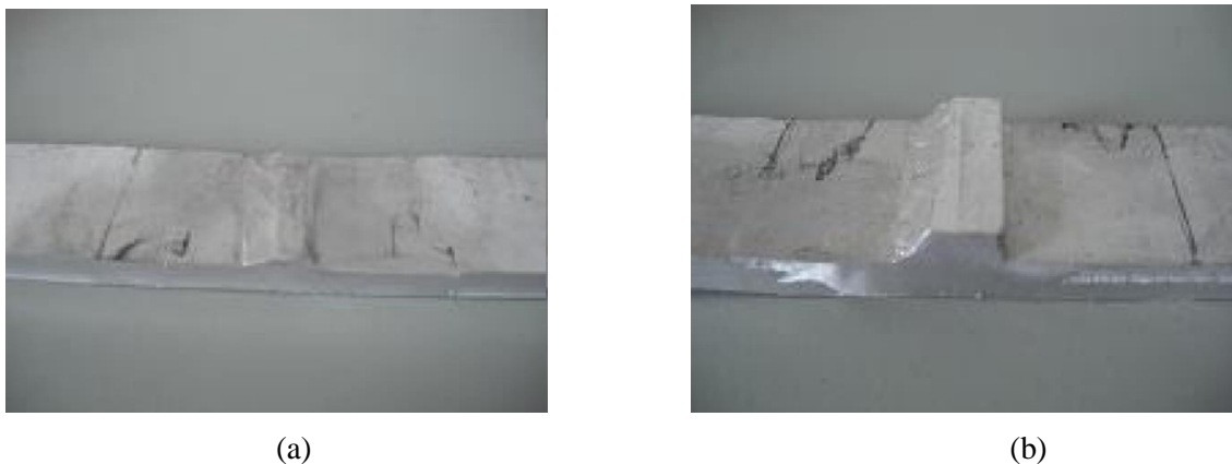
Figure 4. Welded joint test specimens (a) Butt welded joint (b) Fillet welded joint [33] [34]
