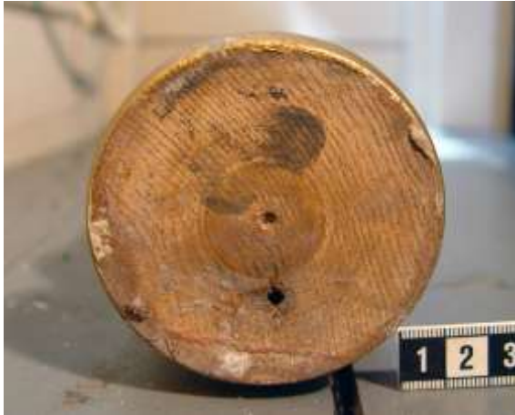
Picture 17 A detail of the column, seen from underneath. A fixing hole from the manufacturing is visible.
