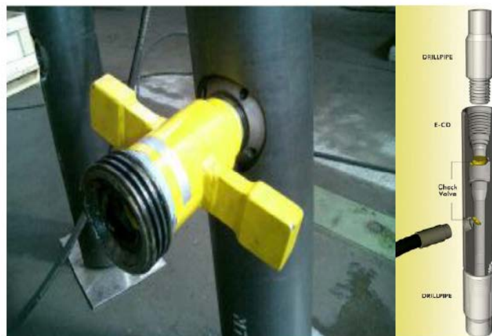
Figure 5.19: continuous Circulation Valve (CCV). (Tercan, 2010)
