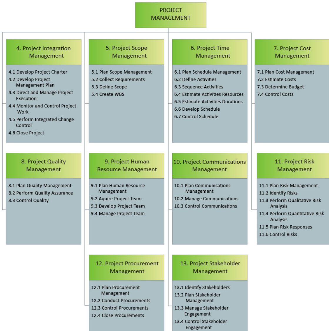
Figure 2. Overview of Project Management Knowledge Areas and Project Management Processes (Metier OEC, 2009, P.8)
