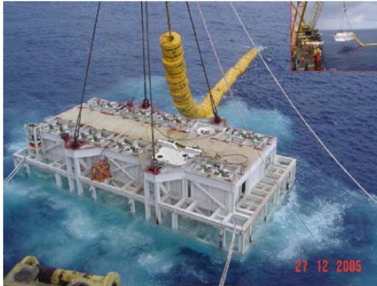
Figure 2.13: Dummy manifold for full-scale test (16.6m*8.5m*5.2m). Courtesy of Petrobras. (He, et al., 2012)
