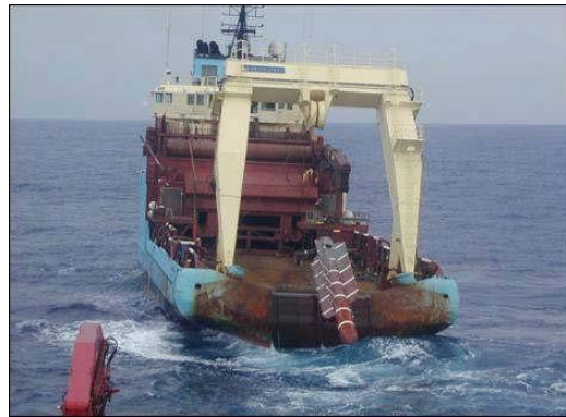
Figure 2.18: Torpedo anchor piles in combination with polyester rope. (He, et al., 2012)
