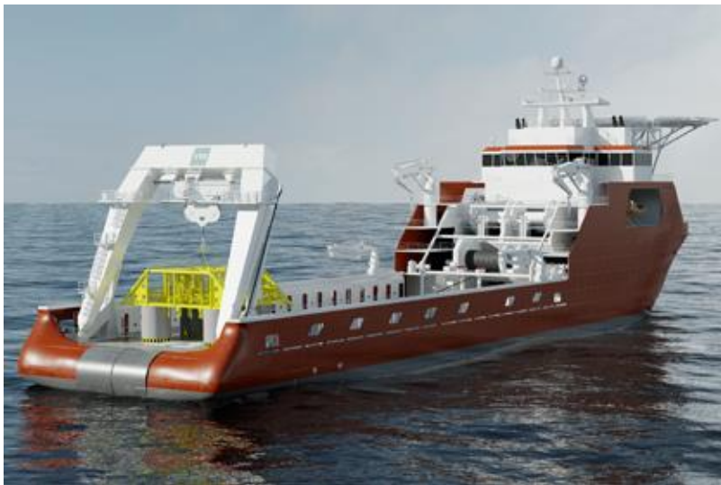
Figure 2.9: AHTS with A-Frame for Manifold Installation. Courtesy of TTS Group ASA. (TTS Group ASA, 2017)
