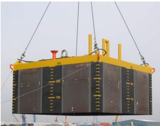
Figure 3.7: Gravity anchors. (Bull, et al., 2007)
