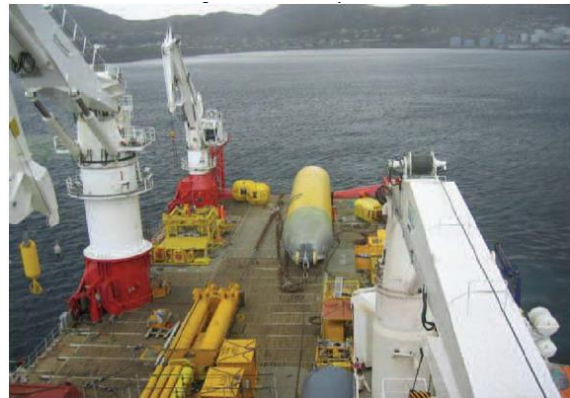
Figure 2.17: Photo of slender Pencil shaped buoy at pre-launch. Courtesy of Aker Solutions.
