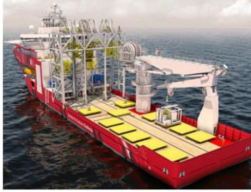
Figure 3.13: Skandi Santos with complete module handling system. (Ingeberg & Torben, 2011)
