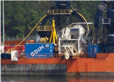
Figure 3.9: FRDS installed on Toisa Perseus. (Bunes, Ingeberg, Torben, & Teigen, 2008)
