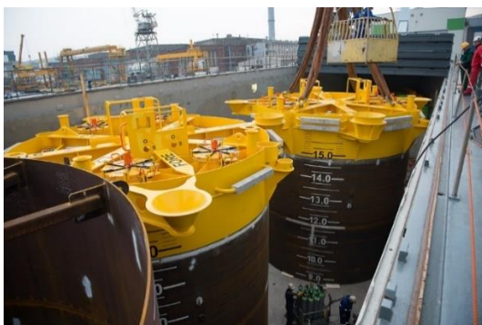
Figure 4.3: Suction anchors. (EPG, 2018)
