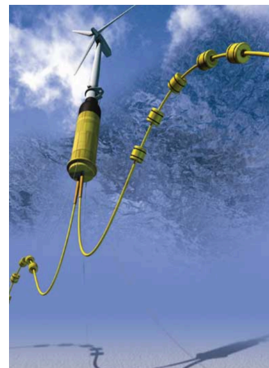
Figure 32: How subsea cables are tied up to the FOWT (PEi, 2010).
