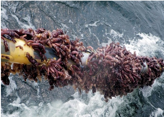
Figure 13: Barnacles on subsea cables (PGS, 2018).
