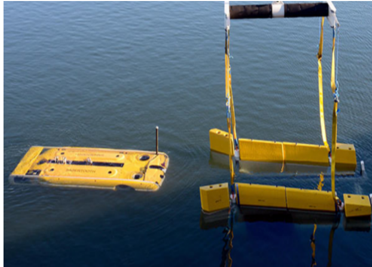
Figure 38: An AUV approaching a docking station (Offshorewind.biz, 2018)
