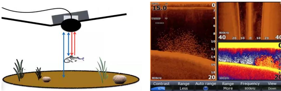
Figure 15 Sonar to detect fish and image from boat adopted from (Kirt Hedquist, 2016)
