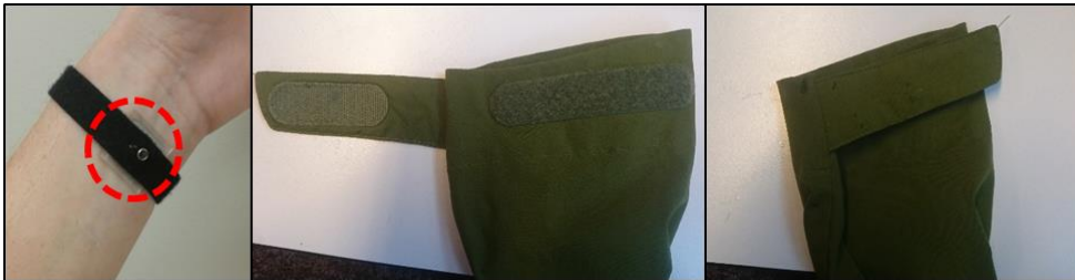
Figure 71 Example of EKG sensor hidden in working clothes / overalls
