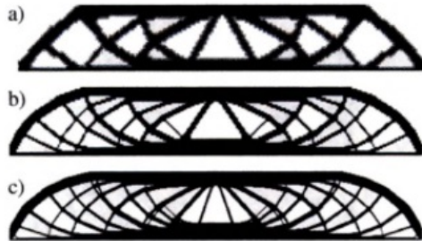
Figure 2.2: Dependence of the optimal topology on mesh refinement for the MBB-beam example. Solution for a discretization with a) 2700, b) 4800 and c) 17200 elements. [10]
