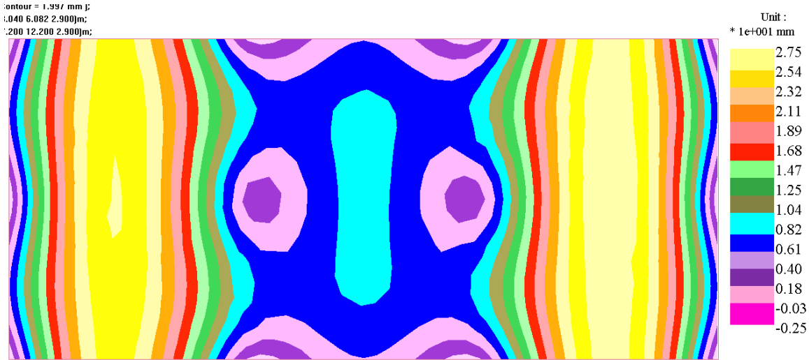
Fig. 4.20 Quasi-Permanent deflections – ADAPT (positive values = downward deflections)
