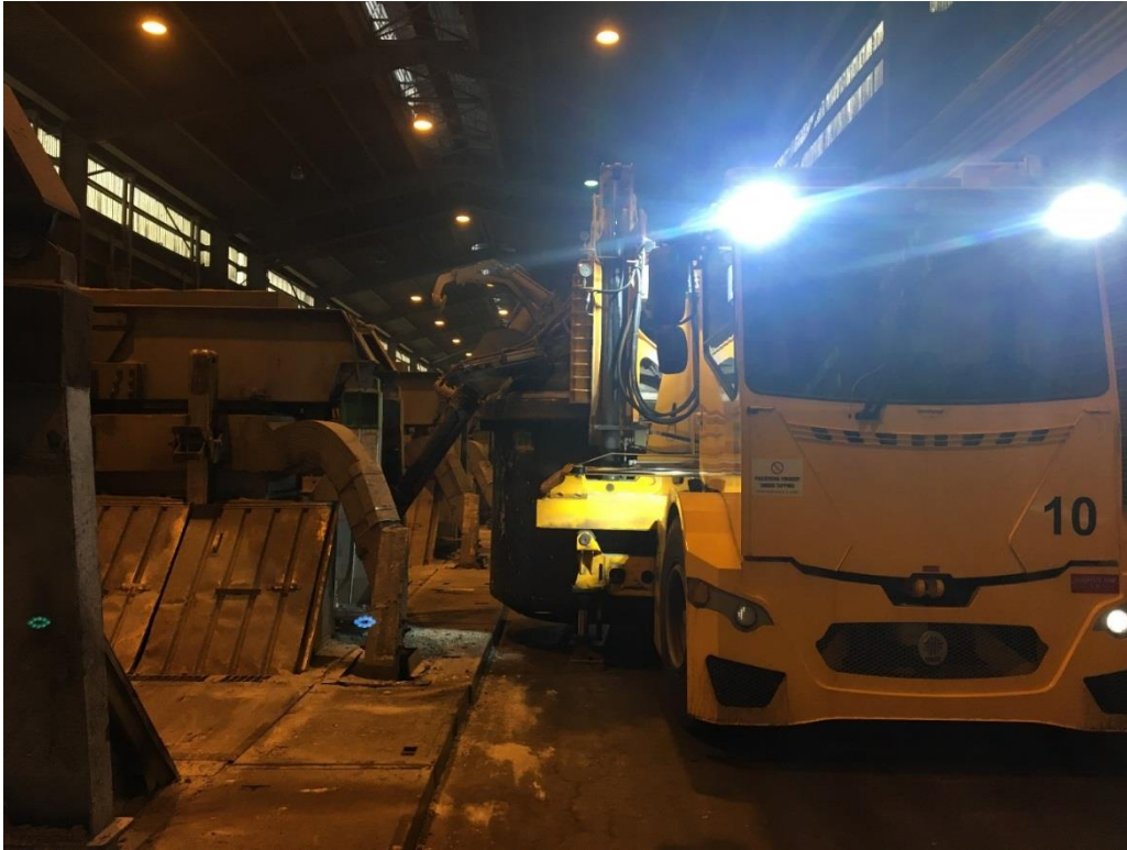
Figure 12: Tapping carriage while tapping aluminium from a cell in Prebake
