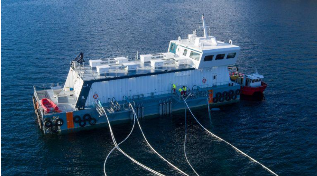
Figure 7: Steinsvik's Nova 600 feed barge with 8 silos and 928 m3 silo capacity (Steinsvik, 2018)
