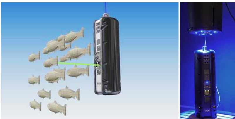
Figure 20: Illustration of Stingray laser node. Photo: Stingray Marine Solutions
