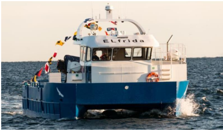
Figure 15: ELFrida, the first electric workboat used in the Norwegian fish farming industry. Image: Enova (Fish farming expert, 2017).
