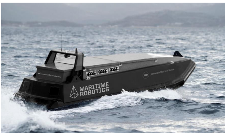
Figure 18: Illustration of an Unmanned Surface Vehicle (USV) carrying ROV and drone (RPAS) between sea cages for various farming operations as inspection, maintenance and repair. Photo: Maritime Robotics (SINTEF, 2016).
