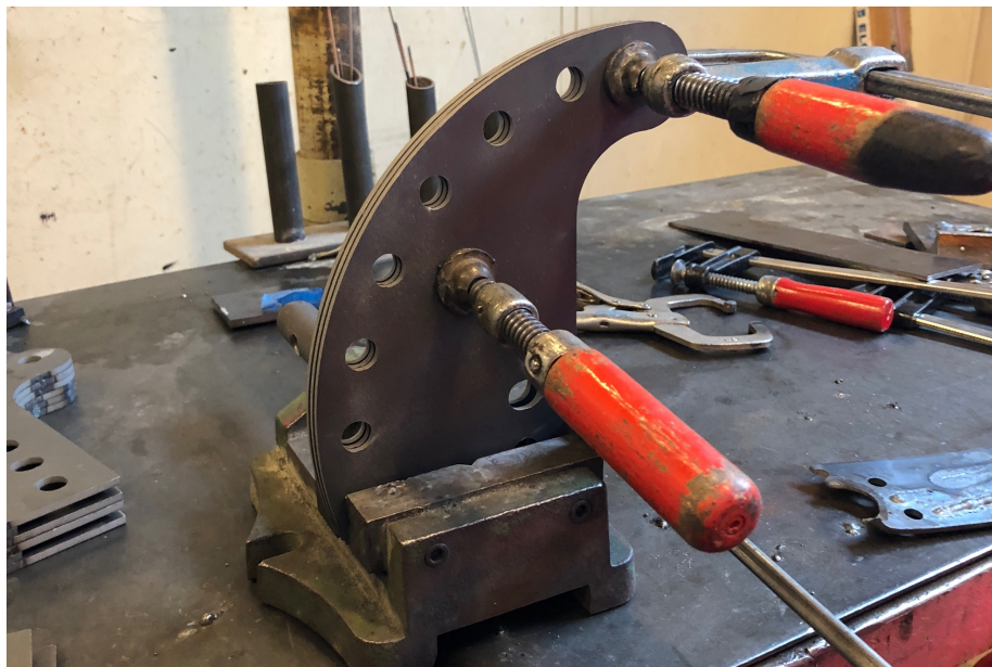
Figure 5-16 Clamping of loading device prior to welding.
