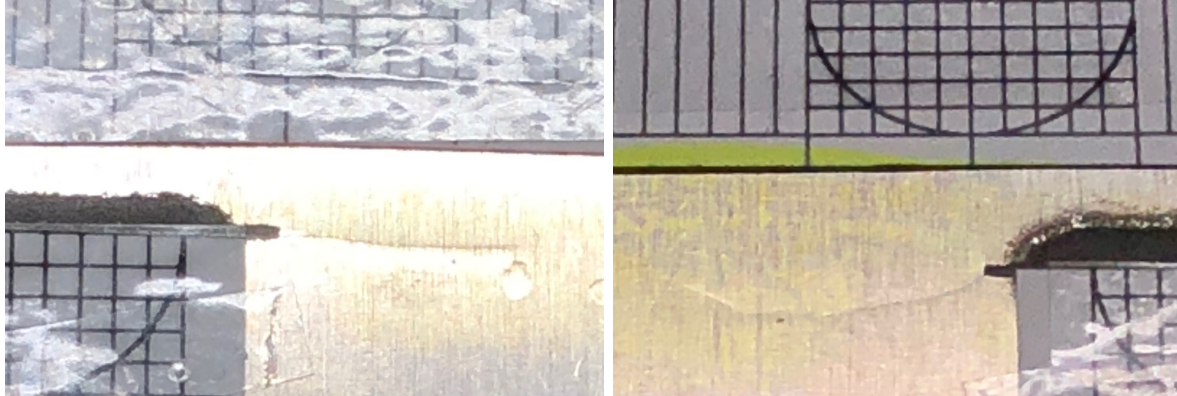
Figure 7-3 Difference in crack growth of the front and the back side during pre-cracking of the third specimen.
