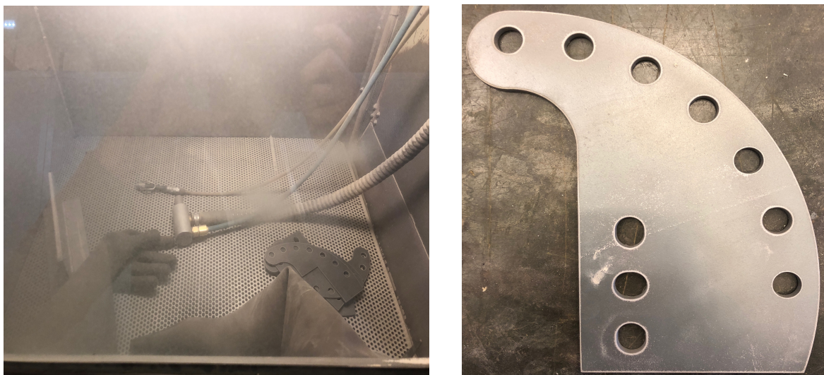
Figure 5-15 Sandblasting of plates before welding.
