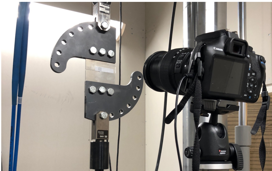
Figure 3-2 Monitoring of crack growth with the use of a photo camera.
