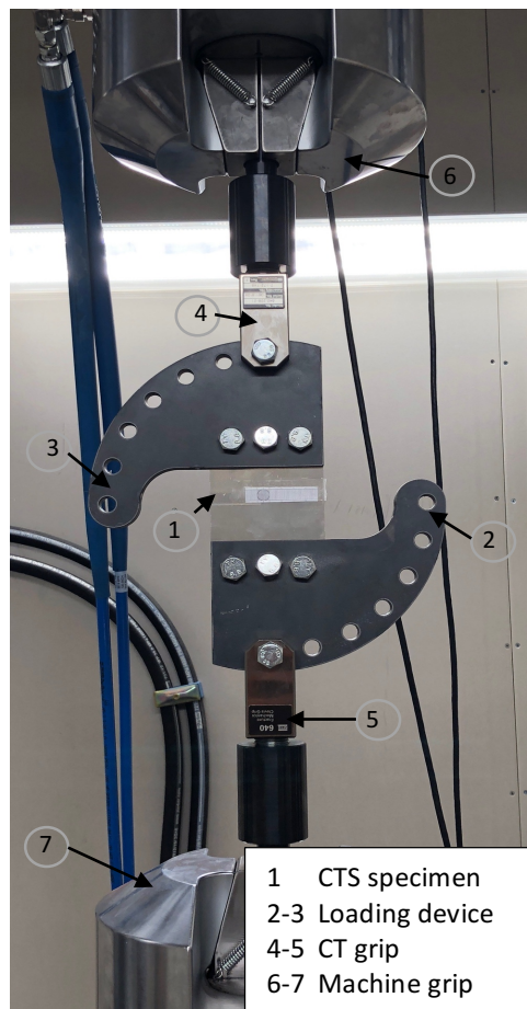
Figure 1-2 Test setup for fatigue test of CTS specimen using designed loading device.
