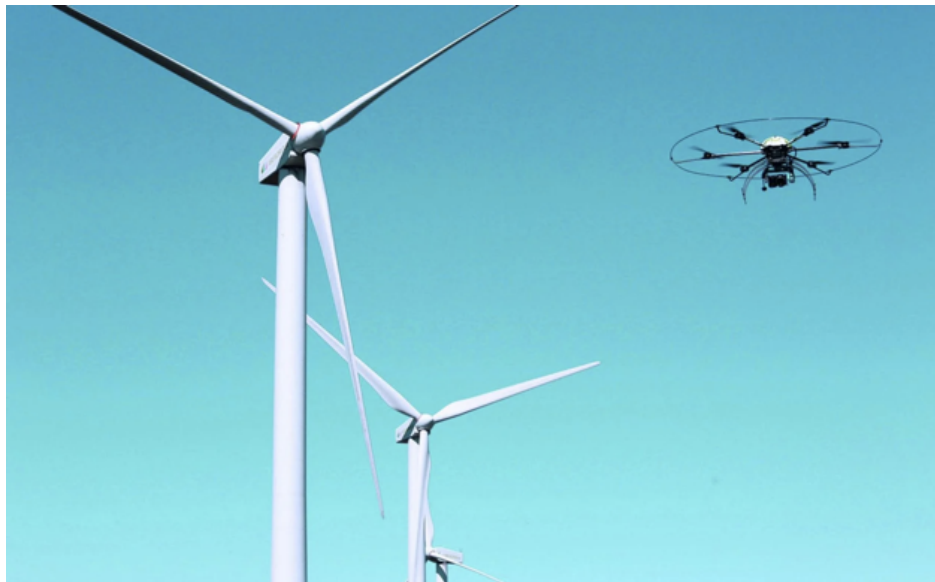
Figure 3-1: Drone used for checking of maintenance conditions of wind turbines (Sucasas, 2018)
