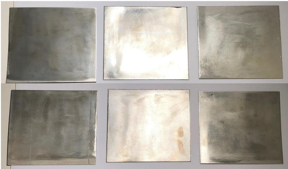
**FIGURE 26:** SAMPLES 3.6.1-3.6.3 EXPOSED SECOND TIME MARINE ATMOSPHERE AND REPASSIVATION.
