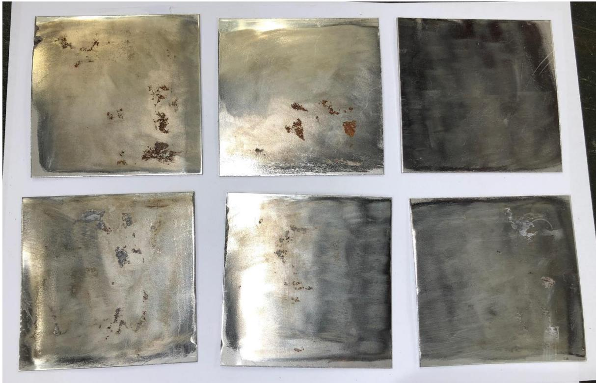
**FIGURE 36:** SAMPLES 2.5.X AND 3.5.X FRONTSIDE APPLIED WITH CORROGEL OFFSHORE.
