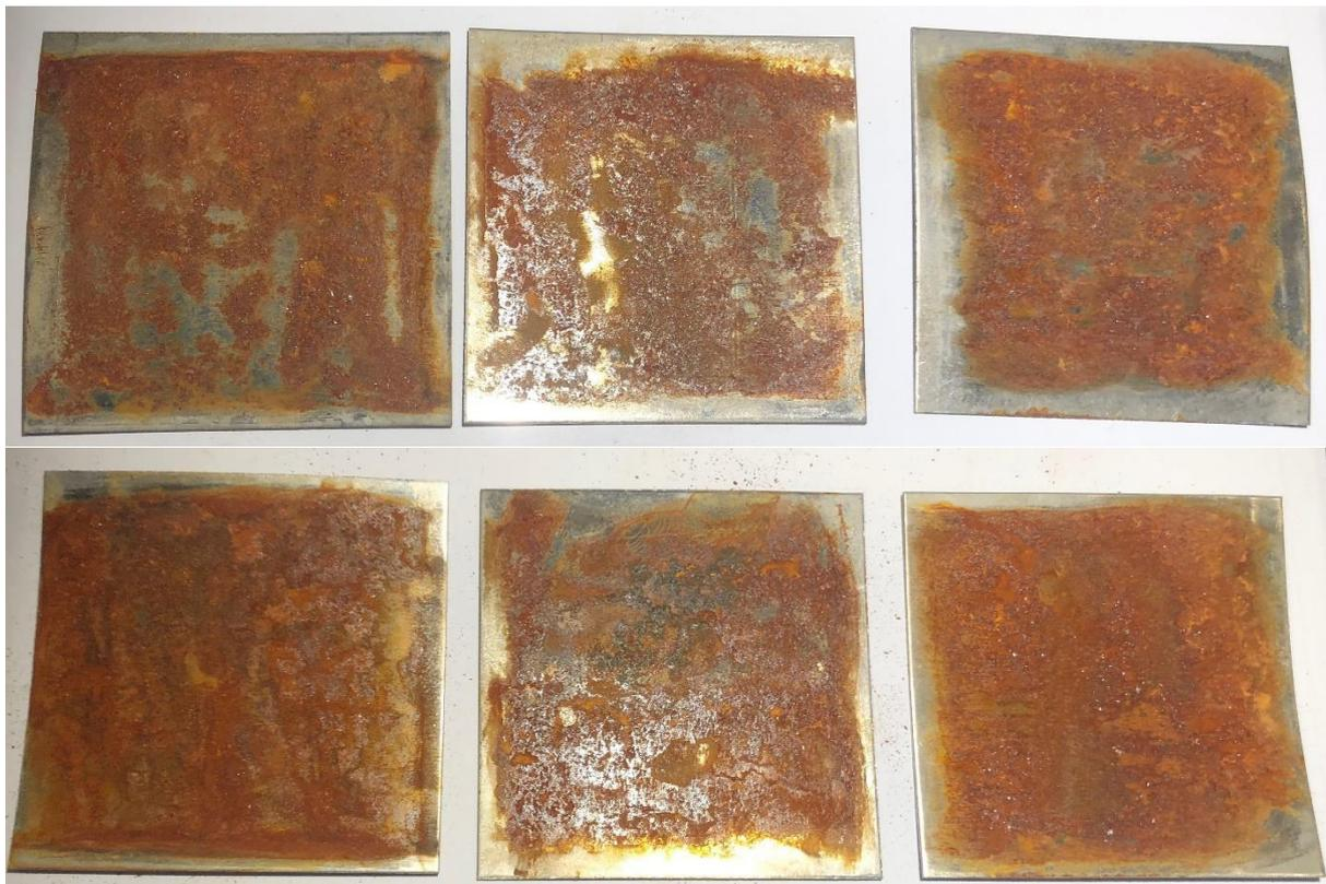
**FIGURE 12:** SAMPLES 3.6.1-3.6.3 FRONTSIDE AND BACKSIDE WERE EXPOSED FOR ROTARY STEEL BRUSH WITH HARD BRAIDED THREADS EQUIPPED BY A GRINDER AND AFTERWARD EXHIBITED FOR MARINE ATMOSPHERE FOR 1 ROUND.
