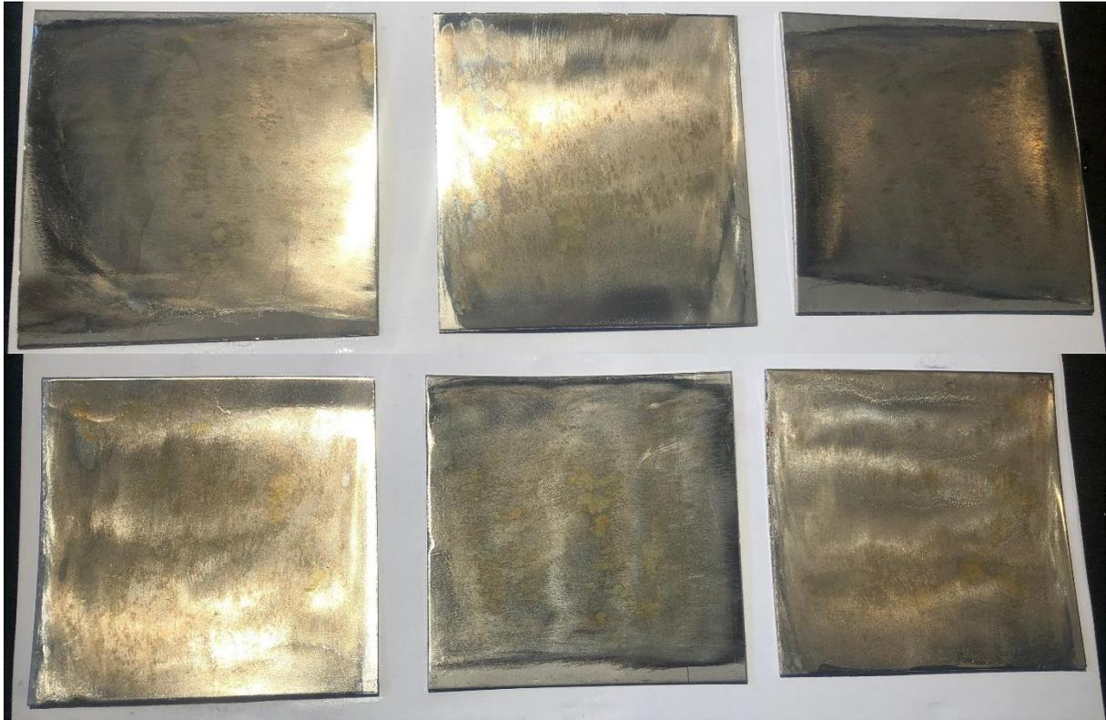
FIGURE 19: SAMPLES 3.4.1-3.4.3 EXPOSED SECOND TIME MARINE ATMOSPHERE AND ONE TIME REPASSIVATION.
