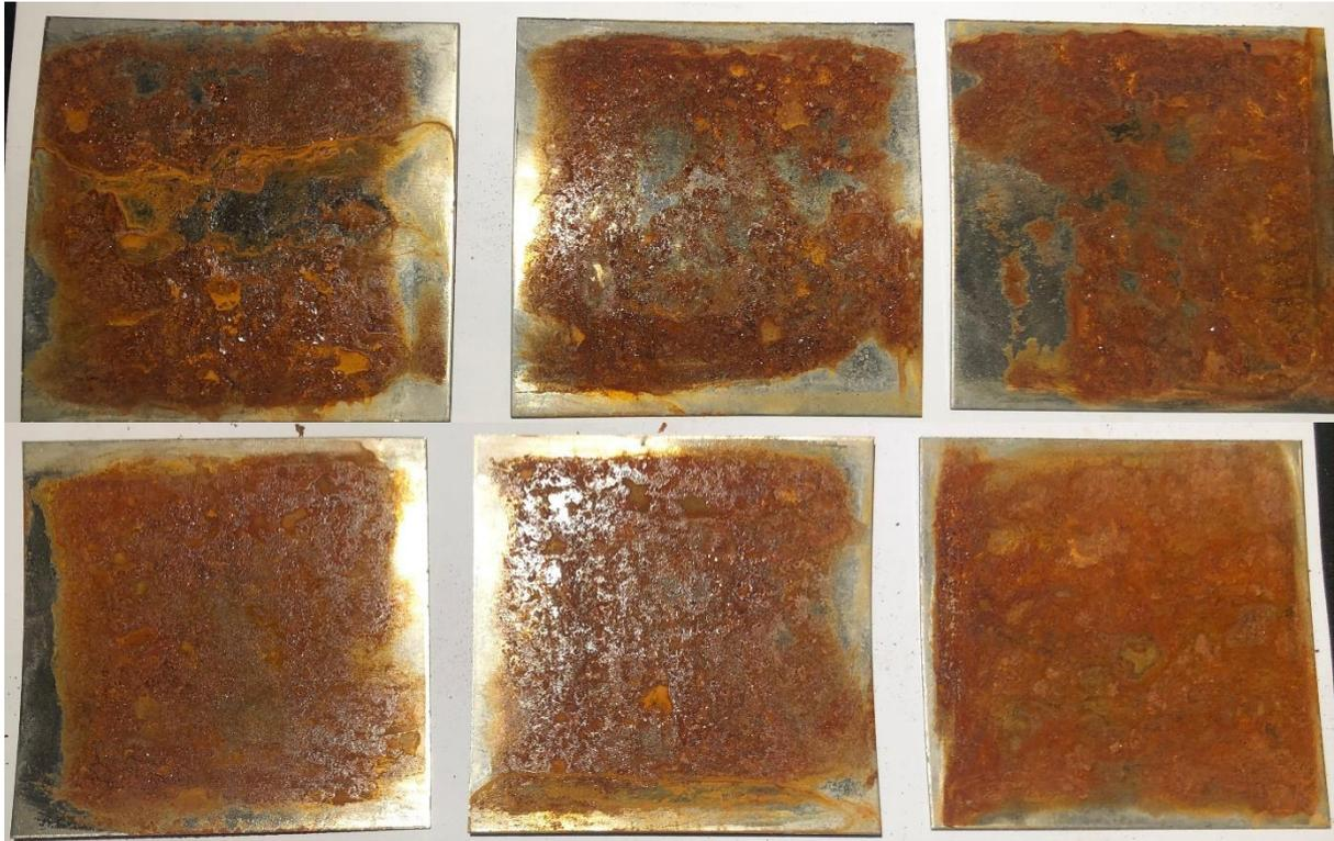
**FIGURE 3:** SAMPLES 2.2.1-2.2.3 FRONTSIDE AND BACKSIDE WERE EXPOSED FOR ROTARY STEEL BRUSH WITH HARD BRAIDED THREADS EQUIPPED BY A GRINDER AND AFTERWARD EXHIBITED FOR MARINE ATMOSPHERE FOR 1 ROUND.
