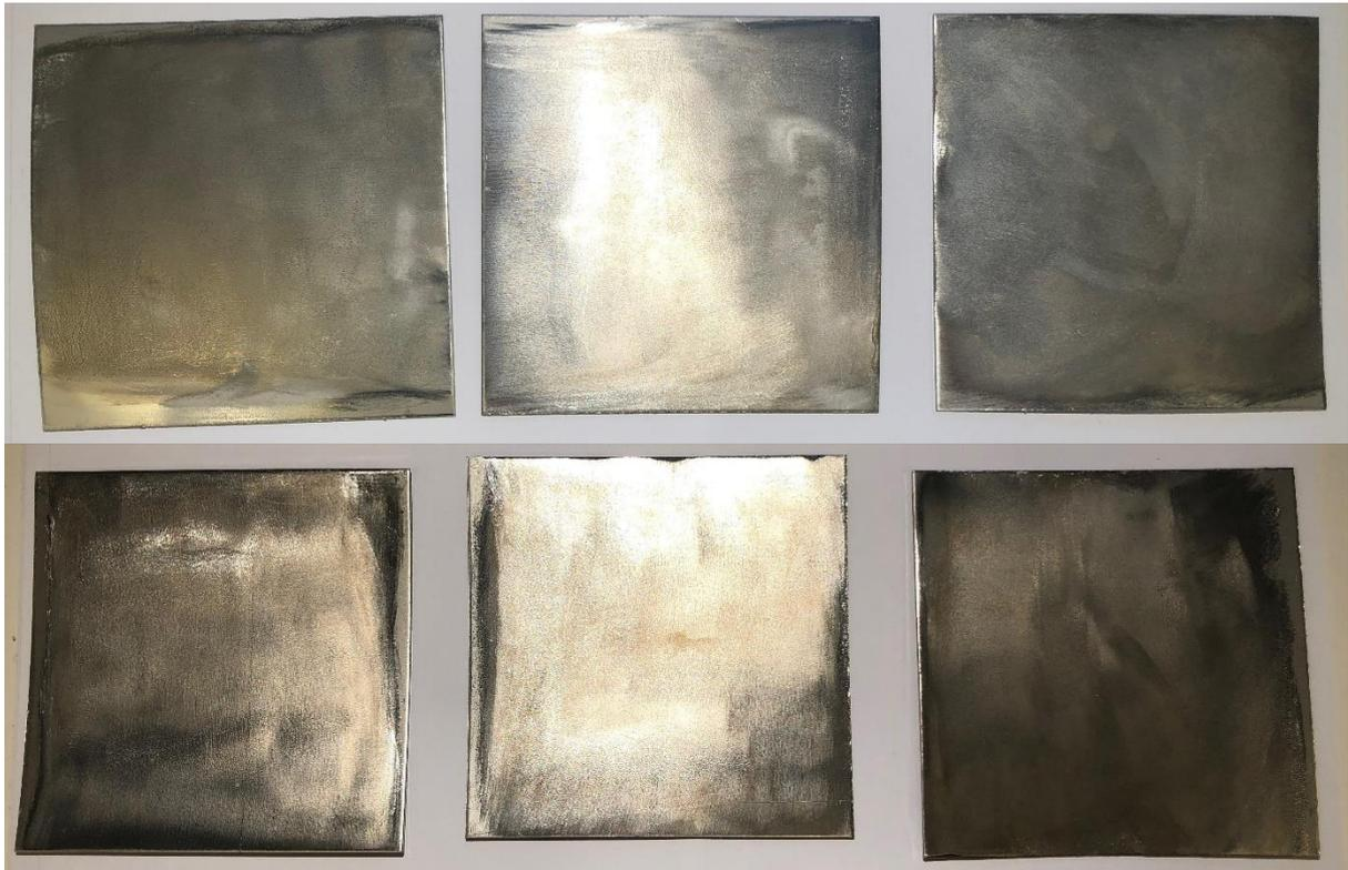
**FIGURE 24: SAMPLES 3.3.1-3.3.3 EXPOSED SECOND TIME MARINE ATMOSPHERE AND REPASSIVATION.**
