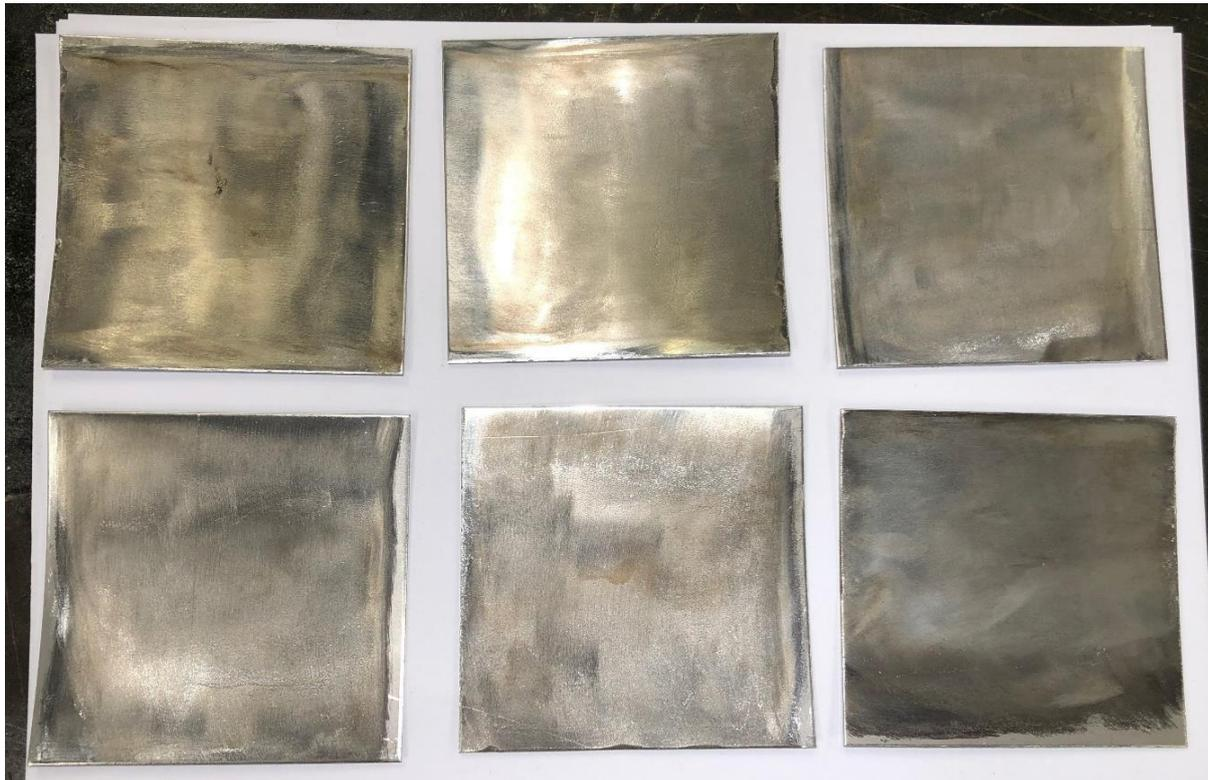
FIGURE 34: SAMPLES 2.3.X AND 3.3.X FRONTSIDE TREATED WITH VALHALL ULTRAGEL.
