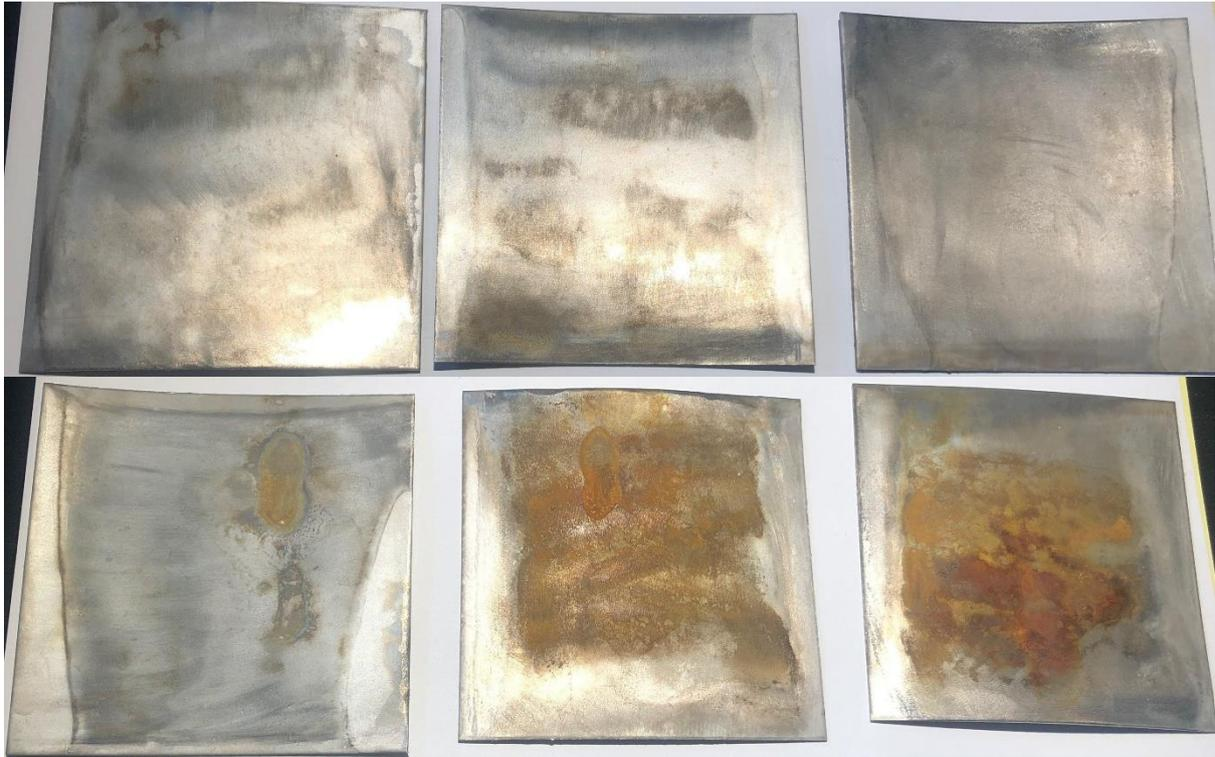
**FIGURE 23: SAMPLES 3.8.1-3.8.3 EXPOSED SECOND TIME MARINE ATMOSPHERE AND ONE TIME REPASSIVATION.**
