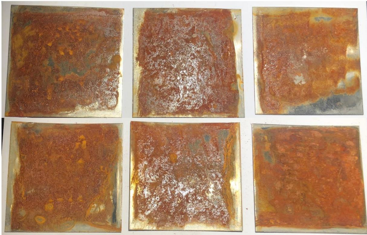
**FIGURE 9:** SAMPLES 2.5.1-2.5.3 FRONTSIDE AND BACKSIDE WERE EXPOSED FOR ROTARY STEEL BRUSH WITH HARD BRAIDED THREADS EQUIPPED BY A GRINDER AND AFTERWARD EXHIBITED FOR MARINE ATMOSPHERE FOR 1 ROUND.
