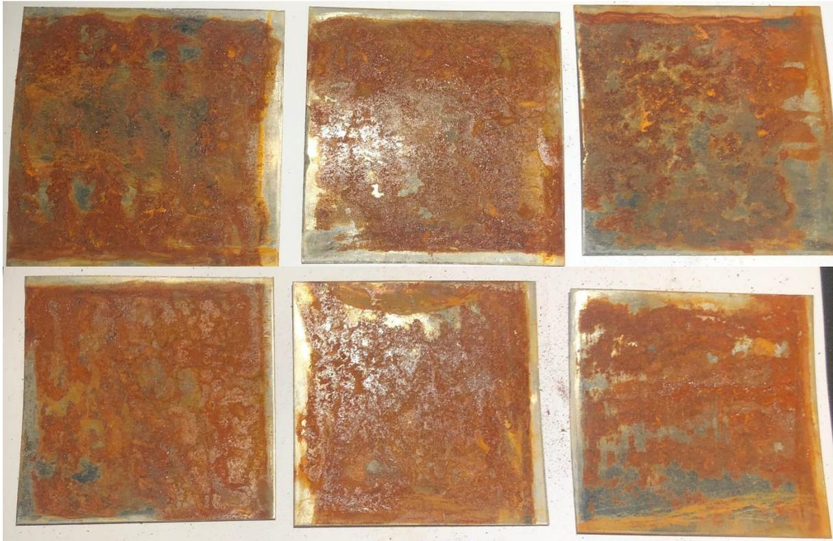
**FIGURE 4:** SAMPLES 3.2.1-3.2.3 FRONTSIDE AND BACKSIDE WERE EXPOSED FOR ROTARY STEEL BRUSH WITH HARD BRAIDED THREADS EQUIPPED BY A GRINDER AND AFTERWARD EXHIBITED FOR MARINE ATMOSPHERE FOR 1 ROUND.
