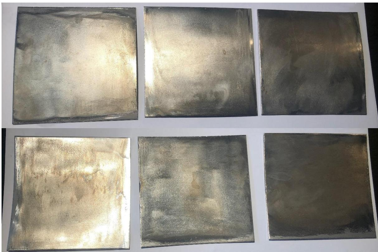
**FIGURE 18:** SAMPLES 3.3.1-3.3.3 EXPOSED SECOND TIME MARINE ATMOSPHERE AND ONE TIME REPASSIVATION.
