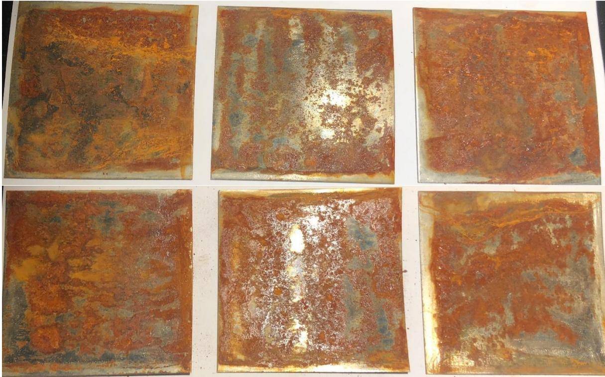
**FIGURE 5:** SAMPLES 2.3.1-2.3.3 FRONTSIDE AND BACKSIDE WERE EXPOSED FOR ROTARY STEEL BRUSH WITH HARD BRAIDED THREADS EQUIPPED BY A GRINDER AND AFTERWARD EXHIBITED FOR MARINE ATMOSPHERE FOR 1 ROUND.
