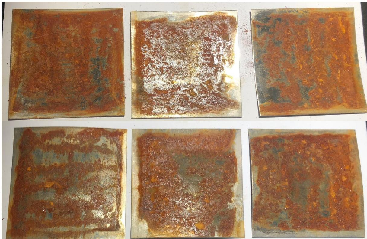
**FIGURE 8:** SAMPLES 3.4.1-3.4.3 FRONTSIDE AND BACKSIDE WERE EXPOSED FOR ROTARY STEEL BRUSH WITH HARD BRAIDED THREADS EQUIPPED BY A GRINDER AND AFTERWARD EXHIBITED FOR MARINE ATMOSPHERE FOR 1 ROUND.
