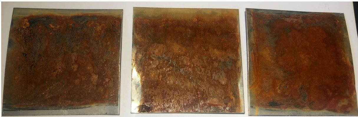
**FIGURE 41:** SAMPLES 3.1.X EXPOSED SECOND TIME FOR MARINE ATMOSPHERE.
