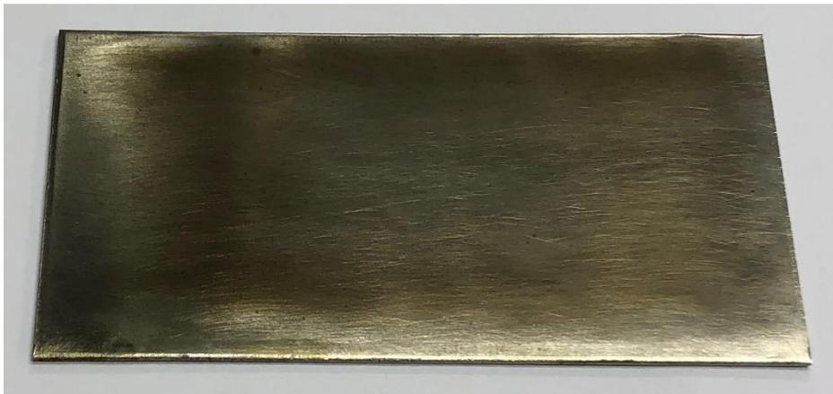
**FIGURE 26:** SAMPLE 0.4 EXPOSED BY A ROTARY STEEL BRUSH WITH SOFT THREADS EQUIPPED ON A BATTERY OPERATED DRILL AND EXHIBITED BY SEAWATER.
