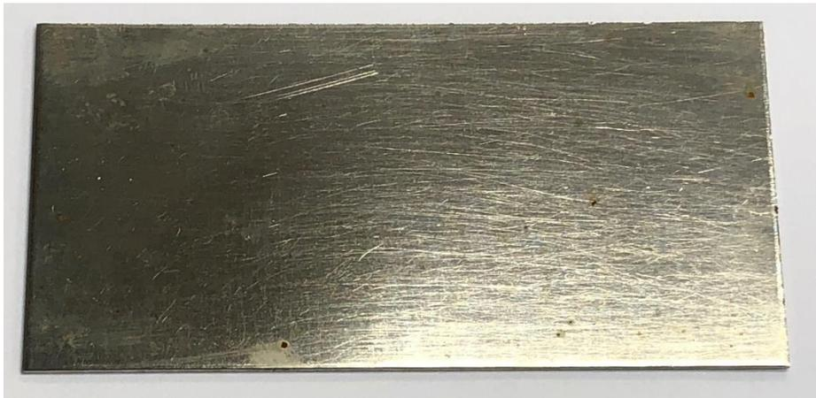
**FIGURE 24:** SAMPLE 0.2 AFTER DAMAGED BY A STEEL BRUSH AND EXHIBITED BY SEAWATER.
