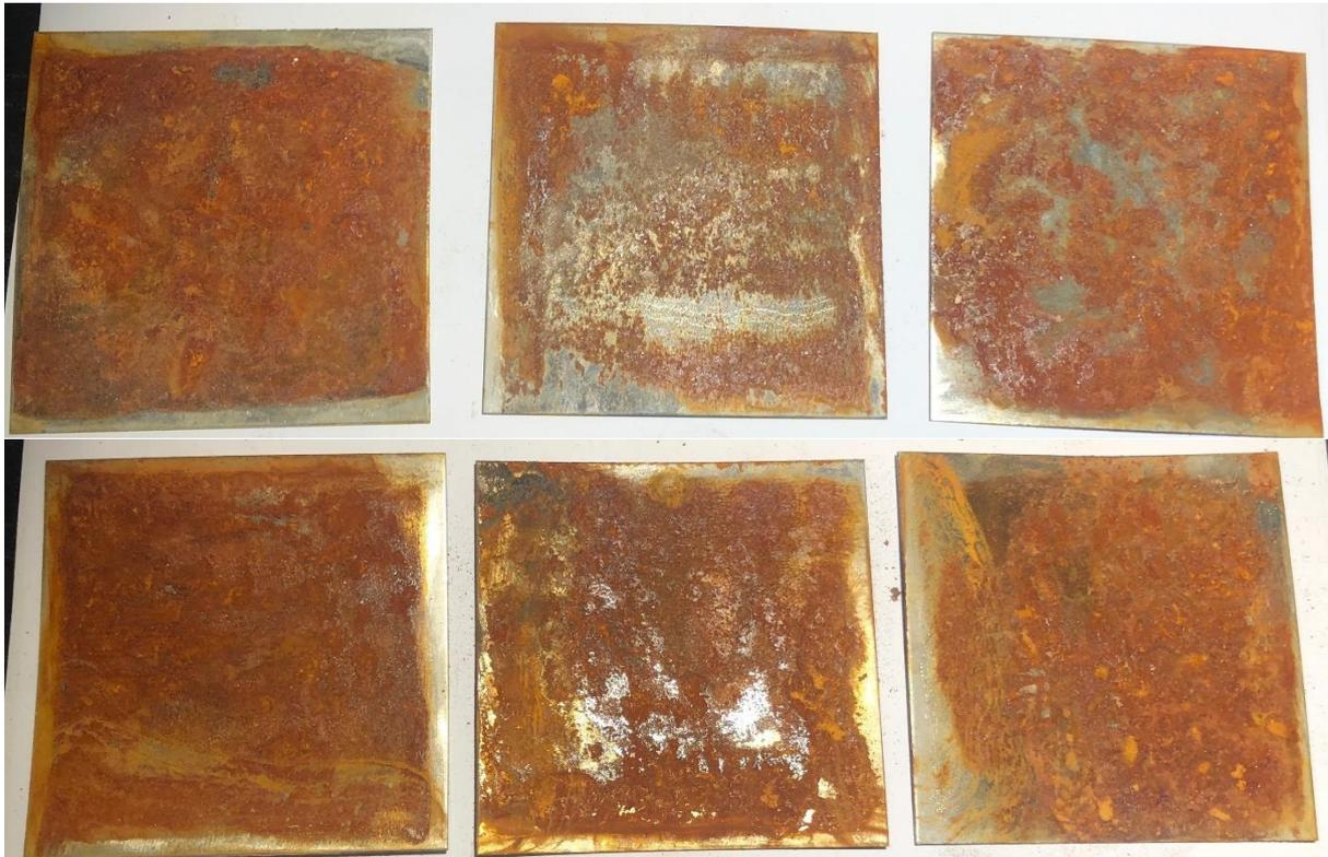
**FIGURE 6:** SAMPLES 3.3.1-3.3.3 FRONTSIDE AND BACKSIDE WERE EXPOSED FOR ROTARY STEEL BRUSH WITH HARD BRAIDED THREADS EQUIPPED BY A GRINDER AND AFTERWARD EXHIBITED FOR MARINE ATMOSPHERE FOR 1 ROUND.
