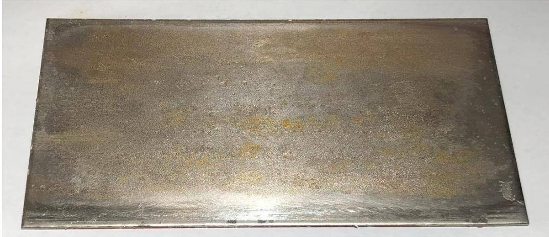
**FIGURE 27:** SAMPLE 0.5 EXPOSED BY A ROTARY STEEL BRUSH WITH SOFT THREADS EQUIPPED ON A HIGH-SPEED AIR COMPRESSOR EXHIBITED BY SEAWATER AND MARINE ATMOSPHERE.
