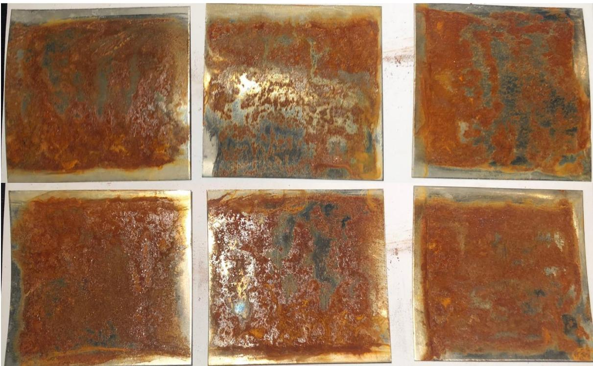
**FIGURE 2:** SAMPLES 3.1.1-3.1.3 FRONTSIDE AND BACKSIDE WERE EXPOSED FOR ROTARY STEEL BRUSH WITH HARD BRAIDED THREADS EQUIPPED BY A GRINDER AND AFTERWARD EXHIBITED FOR MARINE ATMOSPHERE FOR 1 ROUND.
