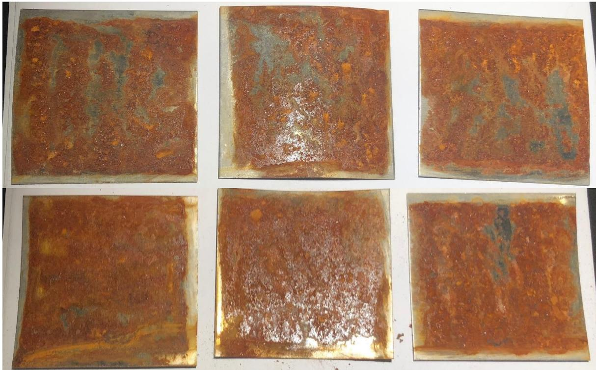
**FIGURE 13:** SAMPLES 2.7.1-2.7.3 FRONTSIDE AND BACKSIDE WERE EXPOSED FOR ROTARY STEEL BRUSH WITH HARD BRAIDED THREADS EQUIPPED BY A GRINDER AND AFTERWARD EXHIBITED FOR MARINE ATMOSPHERE FOR 1 ROUND.
