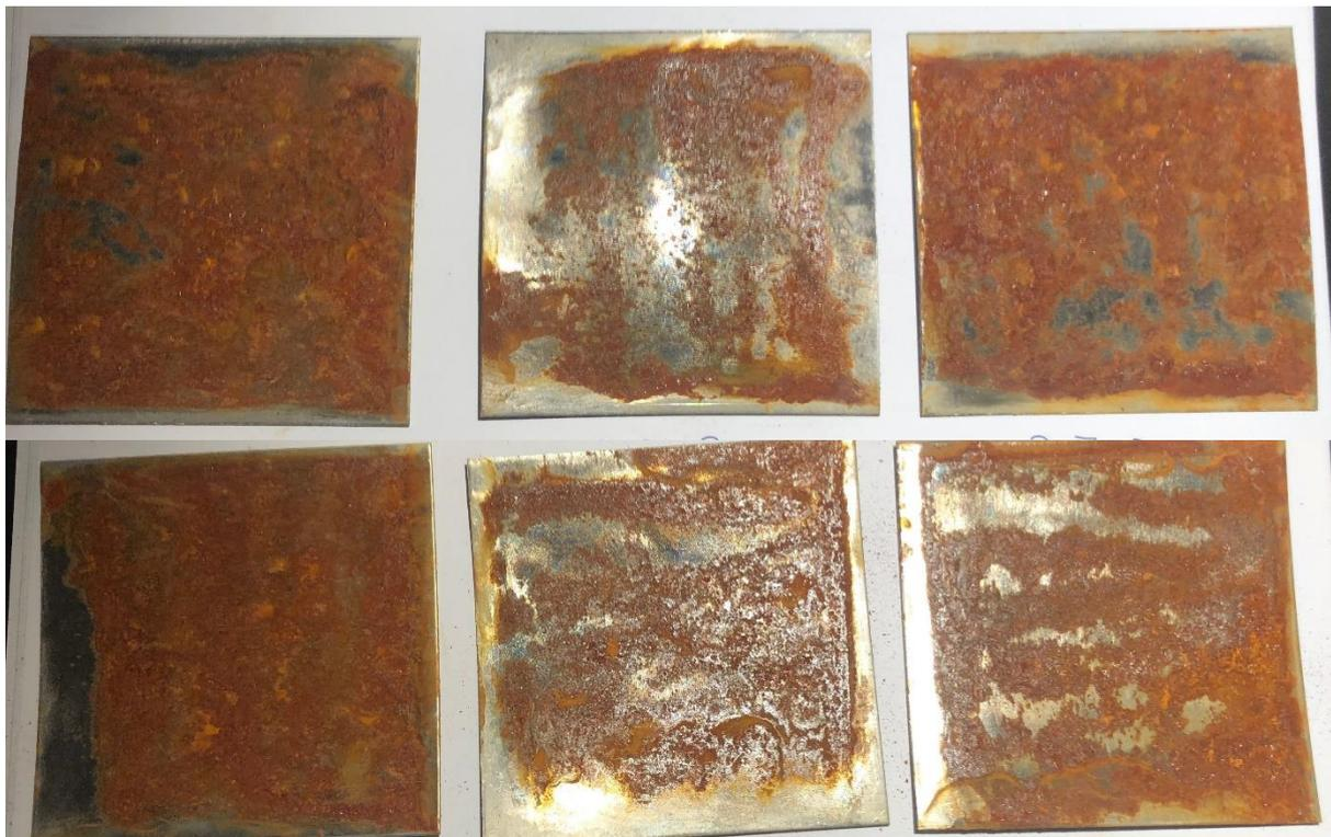
**FIGURE 14:** SAMPLES 3.7.1-3.7.3 FRONTSIDE AND BACKSIDE WERE EXPOSED FOR ROTARY STEEL BRUSH WITH HARD BRAIDED THREADS EQUIPPED BY A GRINDER AND AFTERWARD EXHIBITED FOR MARINE ATMOSPHERE FOR 1 ROUND.
