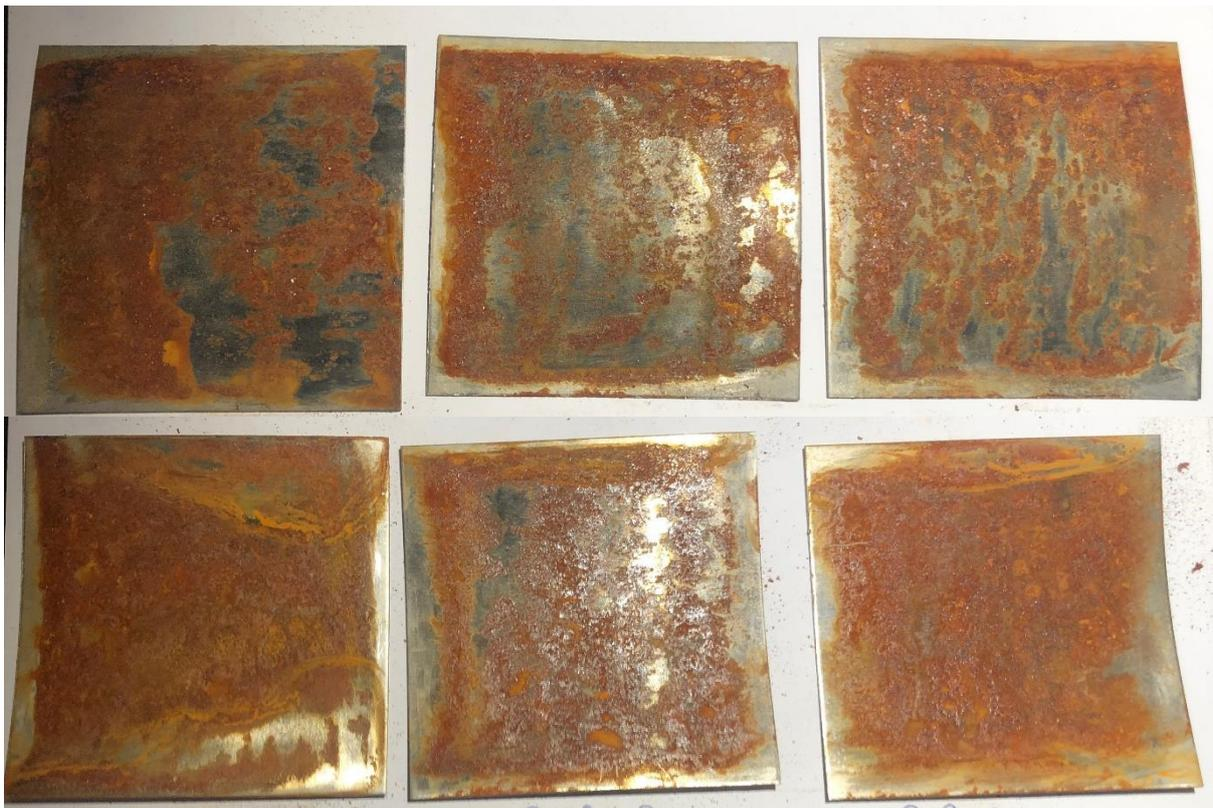
**FIGURE 16:** SAMPLES 3.8.1-3.8.3 FRONTSIDE AND BACKSIDE WERE EXPOSED FOR ROTARY STEEL BRUSH WITH HARD BRAIDED THREADS EQUIPPED BY A GRINDER AND AFTERWARD EXHIBITED FOR MARINE ATMOSPHERE FOR 1 ROUND.
