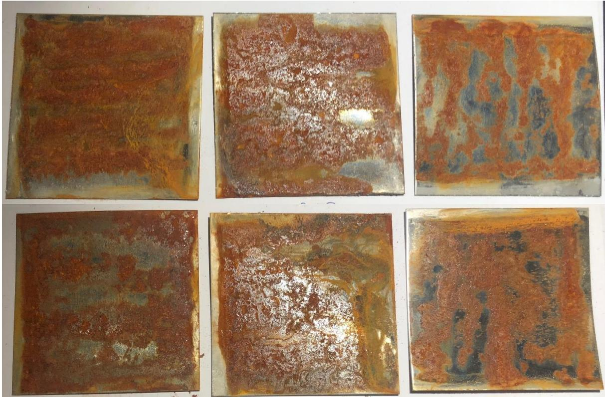
**FIGURE 15:** SAMPLES 2.8.1-2.8.3 FRONTSIDE AND BACKSIDE WERE EXPOSED FOR ROTARY STEEL BRUSH WITH HARD BRAIDED THREADS EQUIPPED BY A GRINDER AND AFTERWARD EXHIBITED FOR MARINE ATMOSPHERE FOR 1 ROUND.
