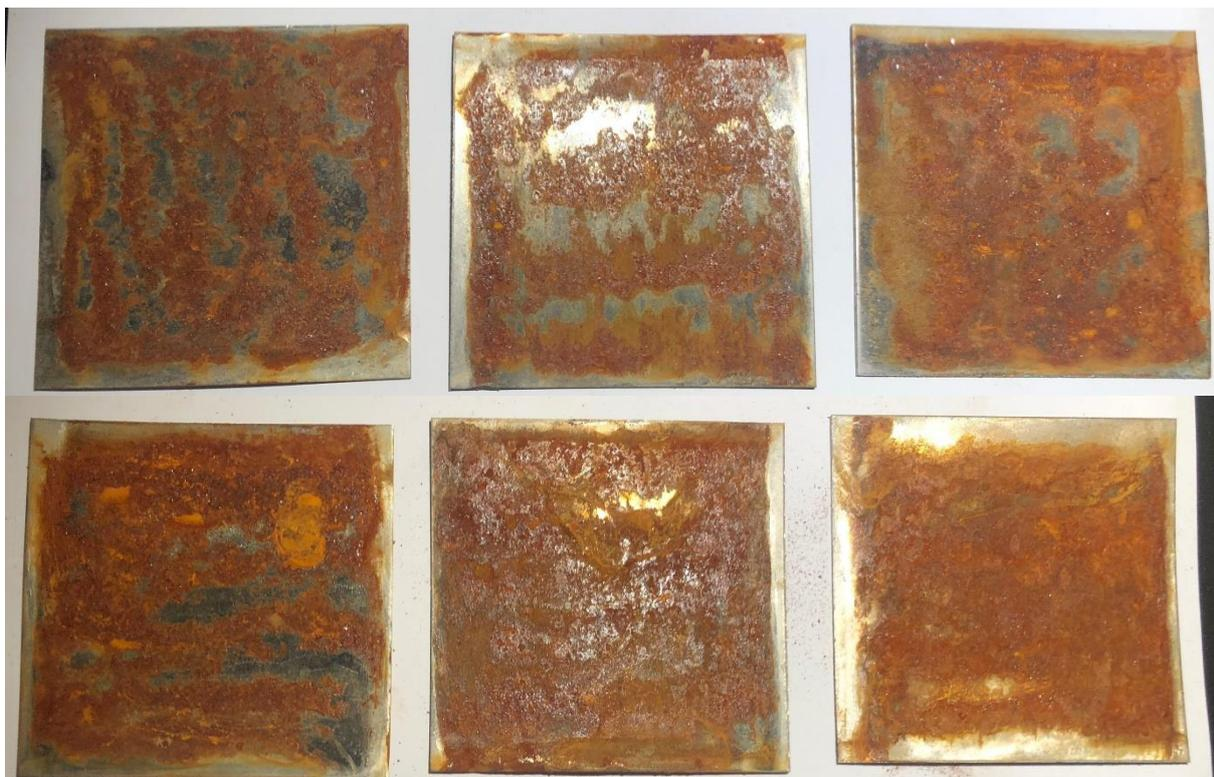
**FIGURE 10:** SAMPLES 3.5.1-3.5.3 FRONTSIDE AND BACKSIDE WERE EXPOSED FOR ROTARY STEEL BRUSH WITH HARD BRAIDED THREADS EQUIPPED BY A GRINDER AND AFTERWARD EXHIBITED FOR MARINE ATMOSPHERE FOR 1 ROUND.
