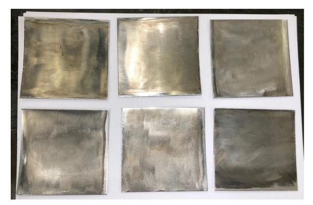
FIGURE 34: SAMPLES 2.3.X AND 3.3.X FRONTSIDE TREATED WITH VALHALL ULTRAGEL.
