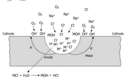
FIGURE 4: PROCESS OF PITTING CORROSION.[9]
