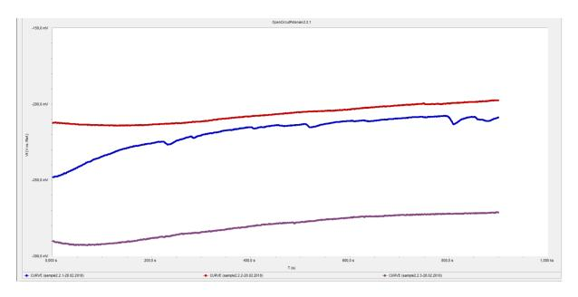
FIGUR 31: SAMPLE 2.2.1-2.2.3 OPEN CIRCUIT POTENTIAL GRAPHS.
