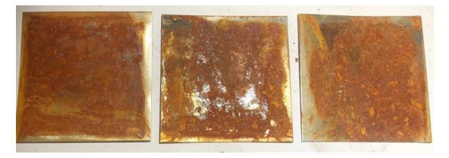
FIGURE 29: SAMPLES EXPOSED FOR GRINDER AND MARINE ATMOSPHERE.
