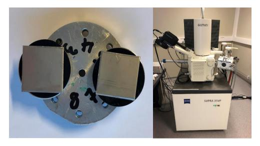
FIGURE 21: SAMPLE A AND B, AND SEM ZEISS SUPRA 35 VP.
