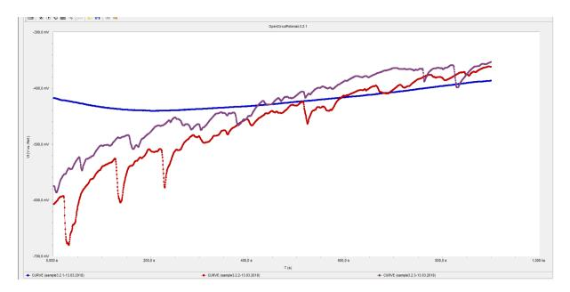
FIGUR 39: SAMPLE 3.2.1-3.2.3 OPEN CIRCUIT POTENTIAL GRAPHS.
