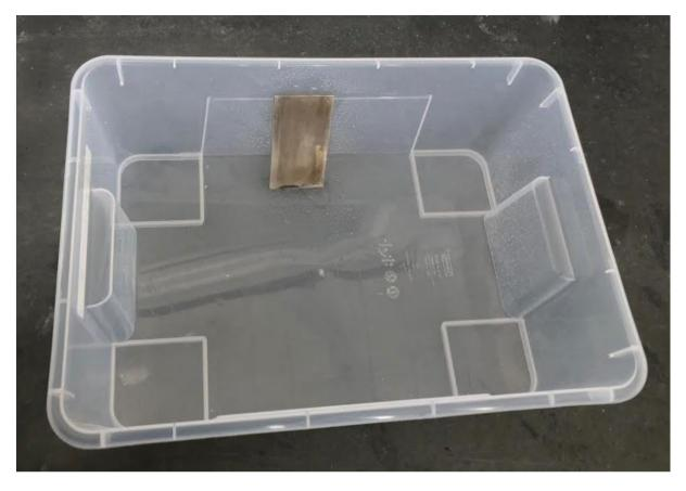
FIGURE 15: SAMPLE 0.5 EXPOSED FOR MARINE ATMOSPHERE.
