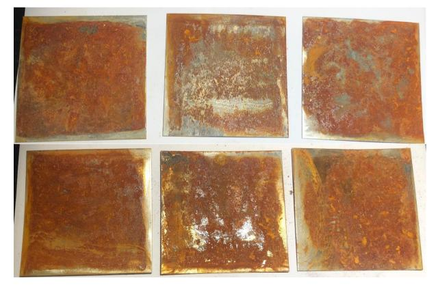
**FIGURE 6:** SAMPLES 3.3.1-3.3.3 FRONTSIDE AND BACKSIDE WERE EXPOSED FOR ROTARY STEEL BRUSH WITH HARD BRAIDED THREADS EQUIPPED BY A GRINDER AND AFTERWARD EXHIBITED FOR MARINE ATMOSPHERE FOR 1 ROUND.
