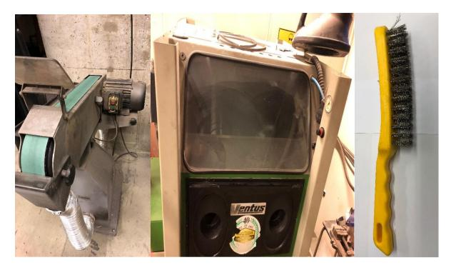
FIGURE 10: LEFT: SANDING BELT, MIDDLE: SANDBLASTER AND RIGHT: WIRE BRUSH.
