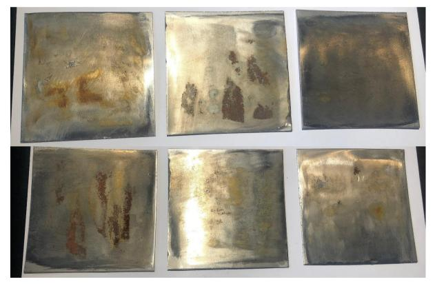
Figure 20: Samples 3.5.1-3.5.3 exposed second time marine atmosphere and one time repassivation.
