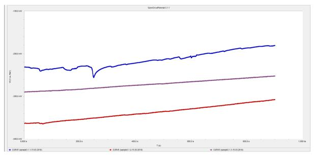
FIGUR 38: SAMPLE 3.1.1-3.1.3 OPEN CIRCUIT POTENTIAL GRAPHS.
