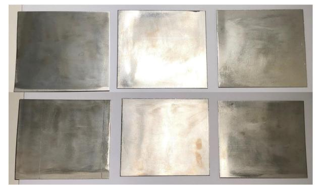
Figure 26: Samples 3.6.1-3.6.3 exposed second time marine atmosphere and repassivation.
