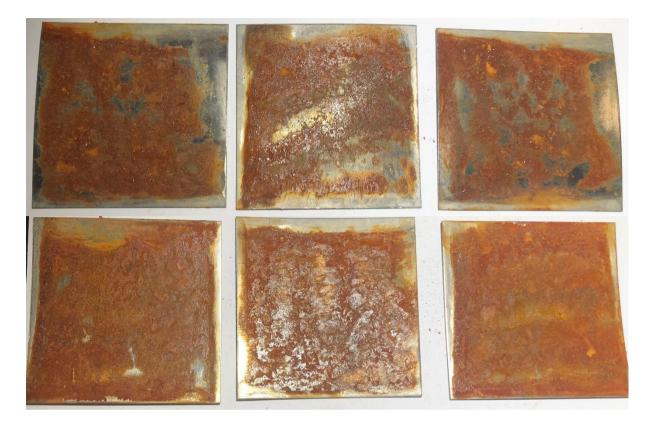
**FIGURE 7:** SAMPLES 2.4.1-2.4.3 FRONTSIDE AND BACKSIDE WERE EXPOSED FOR ROTARY STEEL BRUSH WITH HARD BRAIDED THREADS EQUIPPED BY A GRINDER AND AFTERWARD EXHIBITED FOR MARINE ATMOSPHERE FOR 1 ROUND.
