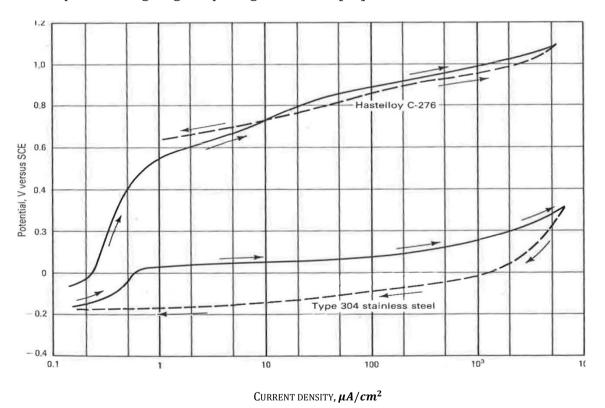
FIGURE 8: POTENTIODYNAMIC CYCLIC POLARIZATION CURVES.[14]
