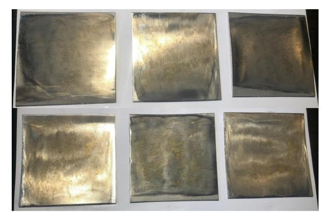
FIGURE 19: SAMPLES 3.4.1-3.4.3 EXPOSED SECOND TIME MARINE ATMOSPHERE AND ONE TIME REPASSIVATION.
