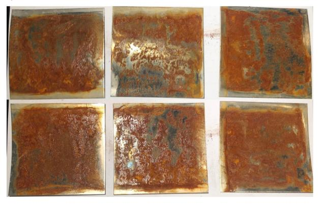
**Figure 2:** Samples 3.1.1-3.1.3 Frontside and backside were exposed for rotary steel brush with hard braided threads equipped by a grinder and afterward exhibited for marine atmosphere for 1 round.
