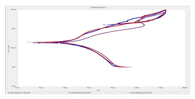
FIGURE 53: CYCLIC POLARIZATION CURVES FOR SAMPLES 2.2.X.
