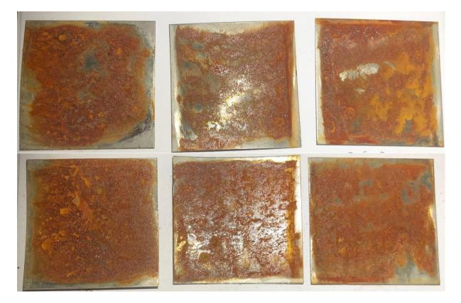
**Figure 11:** Samples 2.6.1-2.6.3 Frontside and backside were exposed for rotary steel brush with hard braided threads equipped by a grinder and afterward exhibited for marine atmosphere for 1 round.
