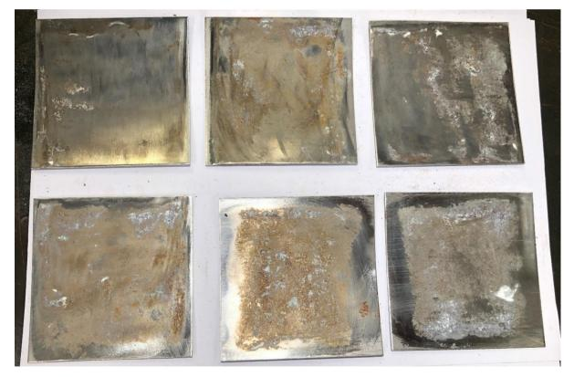
Figure 33: Samples 2.2.X and 3.2.X backside treated with Valhall GreenGel.
