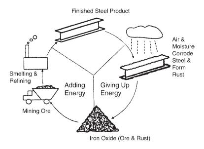
FIGURE 1: CORROSION CYCLE OF STEEL.[8]
