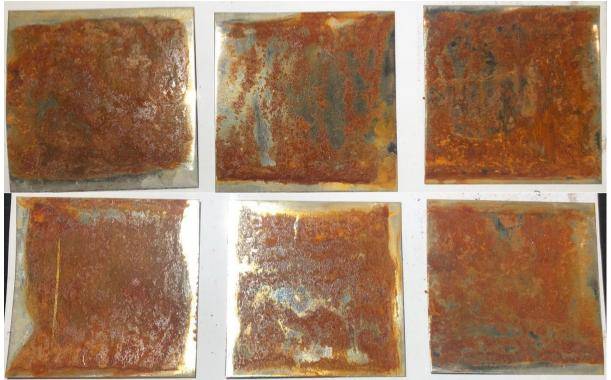
**FIGURE 1:** SAMPLES 2.1.1-2.1.3 FRONTSIDE AND BACKSIDE WERE EXPOSED FOR ROTARY STEEL BRUSH WITH HARD BRAIDED THREADS EQUIPPED BY A GRINDER AND AFTERWARD EXHIBITED FOR MARINE ATMOSPHERE FOR 1 ROUND.
