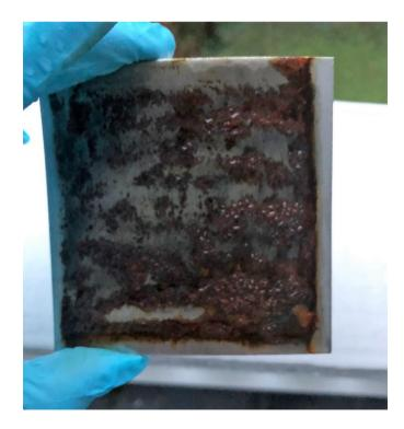
Figure 28: Sample 0.6 exposed by grinder with rotary steel brush with hard braided threads and exhibited for marine atmosphere.
