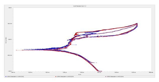
FIGURE 51: CYCLIC POLARIZATION CURVES FOR SAMPLES 1.2.X.
