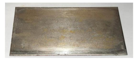
FIGURE 27: SAMPLE 0.5 EXPOSED BY A ROTARY STEEL BRUSH WITH SOFT THREADS EQUIPPED ON A HIGH-SPEED AIR COMPRESSOR EXHIBITED BY SEAWATER AND MARINE ATMOSPHERE.
