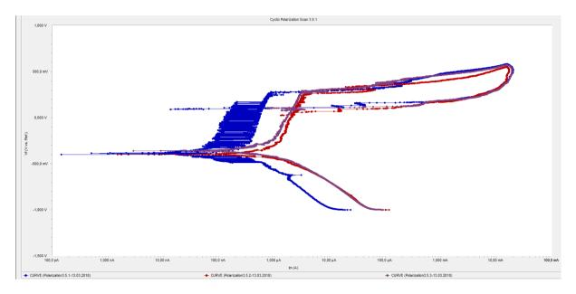
FIGURE 60: CYCLIC POLARIZATION CURVES FOR SAMPLES 3.5.X.
