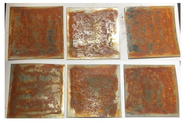
**FIGURE 8:** SAMPLES 3.4.1-3.4.3 FRONTSIDE AND BACKSIDE WERE EXPOSED FOR ROTARY STEEL BRUSH WITH HARD BRAIDED THREADS EQUIPPED BY A GRINDER AND AFTERWARD EXHIBITED FOR MARINE ATMOSPHERE FOR 1 ROUND.
