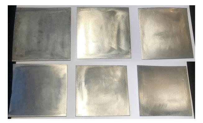
FIGURE 21: SAMPLES 3.6.1-3.6.3 EXPOSED SECOND TIME MARINE ATMOSPHERE AND ONE TIME REPASSIVATION.
