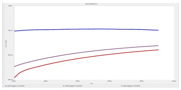
FIGUR 40: SAMPLE 3.3.1-3.3.3 OPEN CIRCUIT POTENTIAL GRAPHS.
