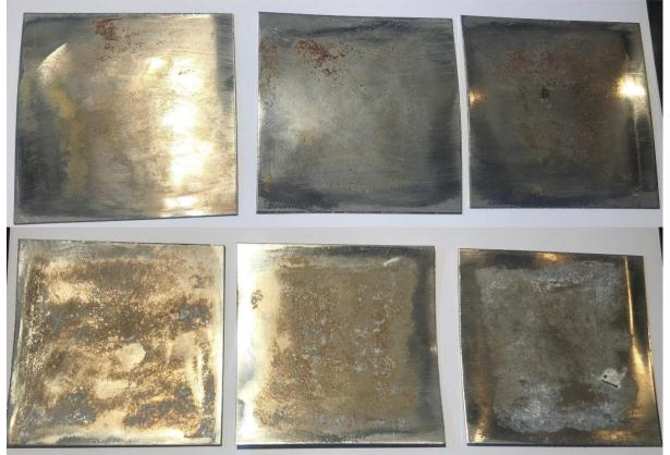
Figure 17: Samples 3.2.1-3.2.3 exposed second time marine atmosphere and one time repassivation.
