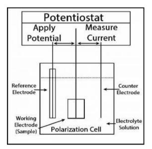
FIGURE 7: SETUP FOR A POLARIZATION CELL.[33]
