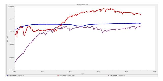
FIGUR 29: SAMPLE 1.3.1-1.3.3 OPEN CIRCUIT POTENTIAL GRAPHS.
