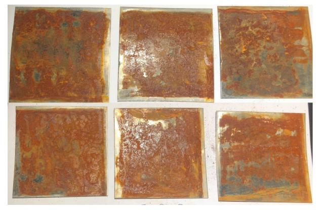
**Figure 4:** Samples 3.2.1-3.2.3 Frontside and backside were exposed for rotary steel brush with hard braided threads equipped by a grinder and afterward exhibited for marine atmosphere for 1 round.
