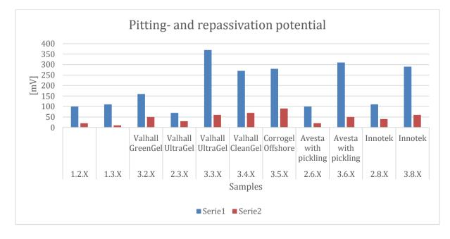
FIGURE 68: REULTS OF PITTING- AND REPASSIVATION POTENTIAL WITHOUT INVALID RESULTS.
