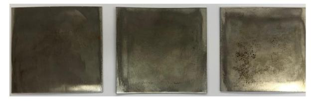
FIGURE 42: SAMPLES 3.2.X AFTER SECOND REPASSIVATION WITH VALHALL GREENGEL.
