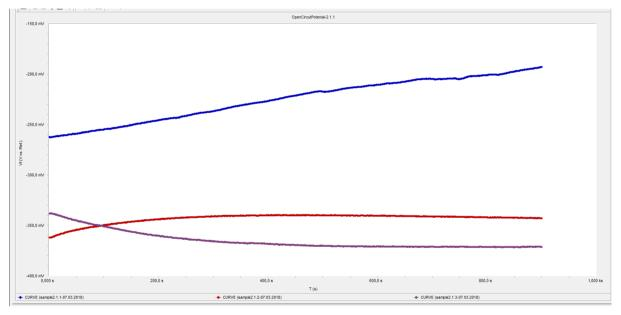
FIGUR 30: SAMPLE 2.1.1-2.1.3 OPEN CIRCUIT POTENTIAL GRAPHS.
