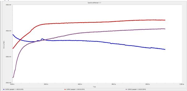
FIGURE 27: SAMPLE 1.1.1-1.1.3 OPEN CIRCUIT POTENTIAL GRAPHS.
