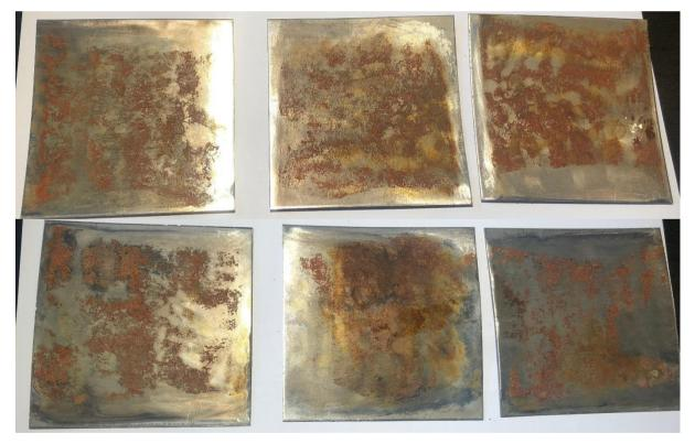
FIGURE 22: SAMPLES 3.7.1-3.7.3 EXPOSED SECOND TIME MARINE ATMOSPHERE AND ONE TIME REPASSIVATION.
