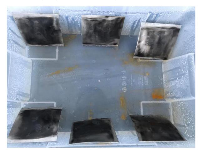
FIGURE 17: SOME SAMPLES EXPOSED FOR MARINE ATMOSPHERE.
