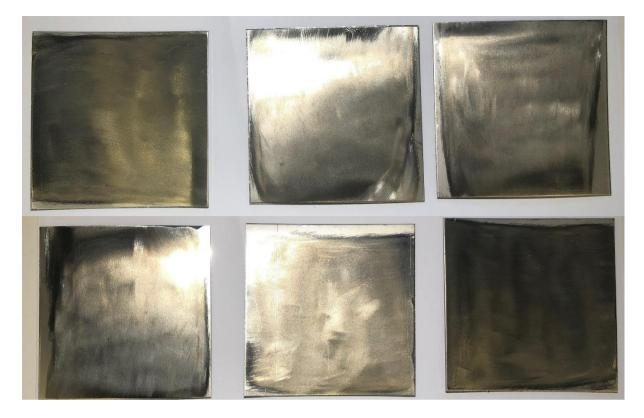
FIGURE 25: SAMPLES 3.4.1-3.4.3 EXPOSED SECOND TIME MARINE ATMOSPHERE AND REPASSIVATION.
