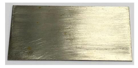
Figure 23: sample 0.1 after been exposed for sanding belt and seawater.
