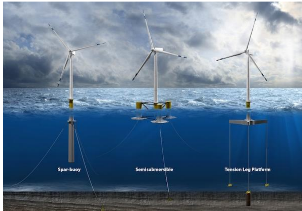
Figure 1.3. Typical concepts of floating wind turbine foundation (Graphic from Josh Bauer, National Renewable Energy Laboratory) [9].
