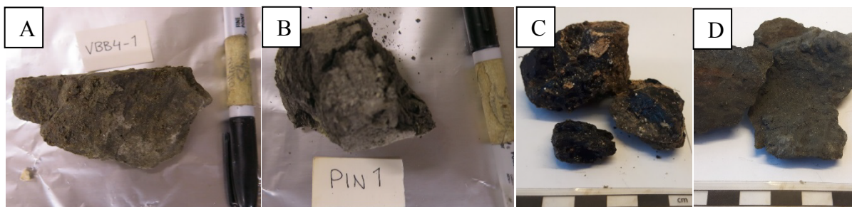
Figure 14 A the oil stained sandstone sample V1 from the well VBB4, B the oil stained siltstone sample collected from the Pindars River BH3 well, C the oil stained carbonate sample D2, E the oil saturated siltstone sample E1.
