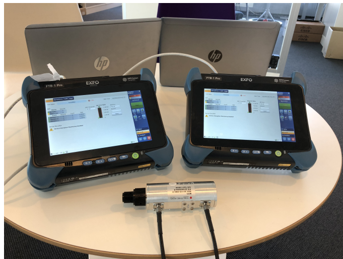
Figure 5.6: Photograph of traffic testers and variable attenuator used for the experiment.
