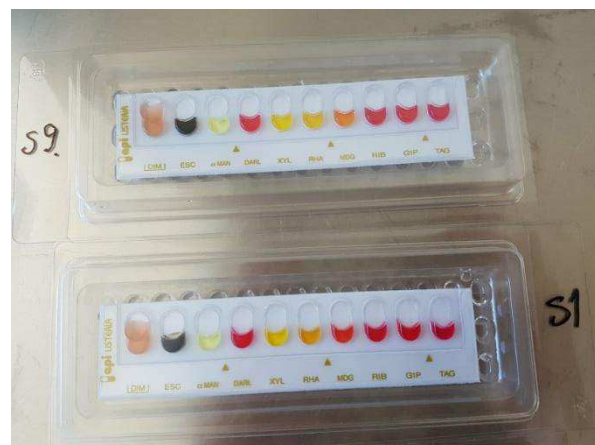
Figure 3.3 API Listeria test for two muscle + skin samples. The positive (s9) and negative reaction (s1) of the MDG well.
