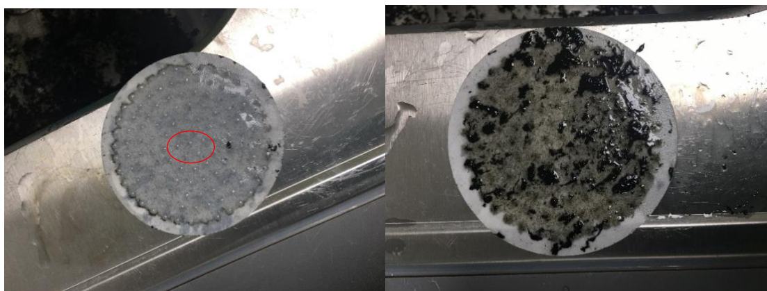
Figure 4.18. Filter damage during Time to filter test.
