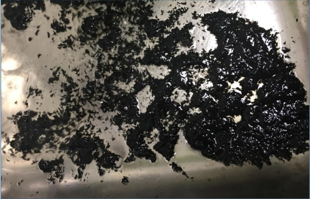
Figure 4.19. Flocs characteristics when obtaining the best dewatering results, when utilizing 100 mL seawater as Mg^{2+} source.
