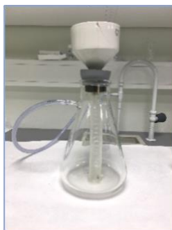
Figure 3.4.3.1. Dewatering test set up.
