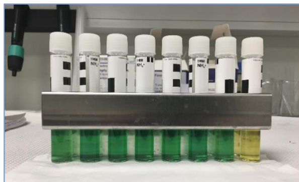
Figure 3.5.3.1 Ammonium cell test.
