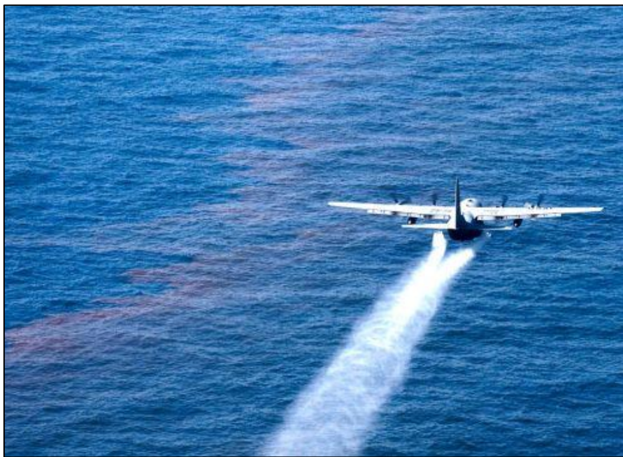
Figure 2.14 Airplane releasing dispersant onto an oil slick on the Gulf of Mexico during the DWH response [12].
