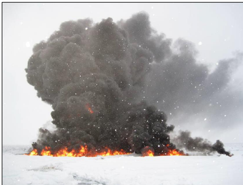
Figure 2.11 In situ burning of weathered free-floating oil in high ice cover during a field experiment in the Barents Sea [8].
