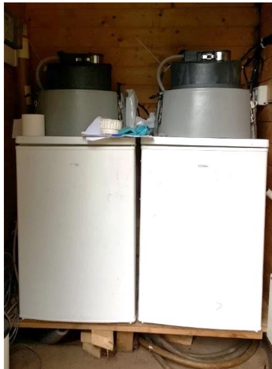
Figure 3-16 The ISCO 6712 Full-Size Portable Samplers placed inside house. Each of the samplers are placed on a refrigerator with the 11 L plastic containers inside.
