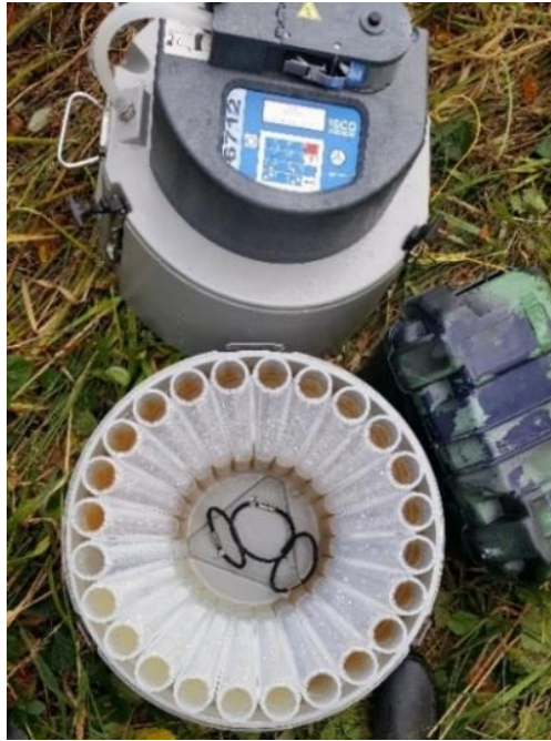
Figure 3-19 Carousel arrangement inside the portable automatic sampler placed at the inlet of pond 1.
