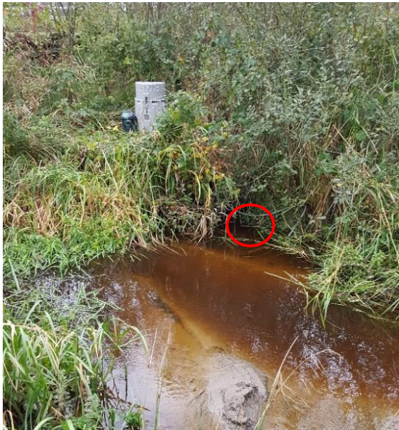
Figure 3-17 The automatic sampler placed over the inlet to pond 1. A car battery was placed with the sampler to provide electricity. The suction tube is marked with a red circle.
