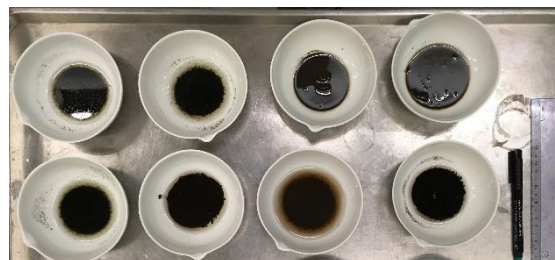
Figure 3.7 Wet sediment samples in porcelain dishes before evaporation.
