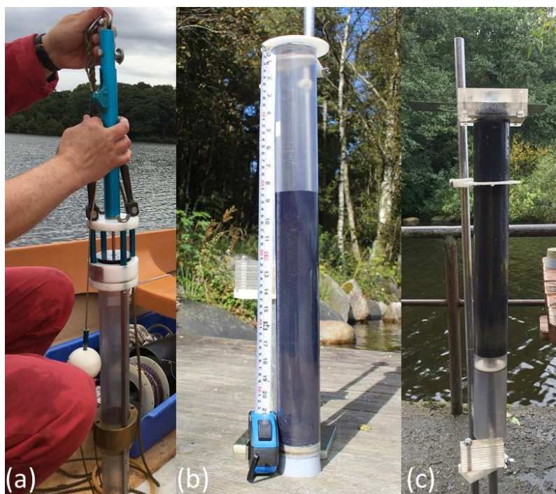
Figure 3.5 Sediment core sampler (a), collected core from Stora Stokkavatnet (b) and vertical extrusion system for the slice and remove sediment section (c).
