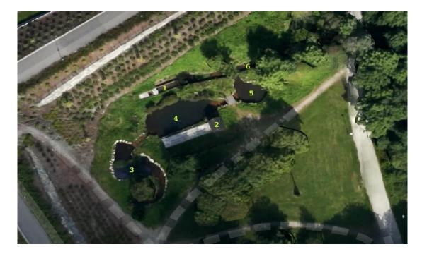
Fig 3-2 Madlabekken constructed wetland (1: Inlet channel, 2: Pump station, 3: planted pond, 4: first sedimentation pond, 5: second sedimentation pond, 6: Outlet channel) (*Photo: Google map*)
