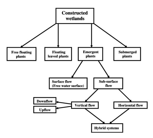
Fig 2-1 Classification of constructed wetlands for wastewater treatment (Vymazal, et al., 2013)
