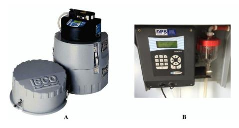
Figure 3-3 Automatic samplers, A. ISCO 6712, B. Sigma max 900
