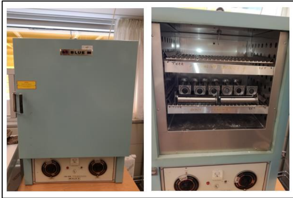
Figure 3-16: Blue M Heat Cabinet in which the cased cement pipes were stored and exposed to temperatures of approximately 110 °C (Aarnes 2018)
