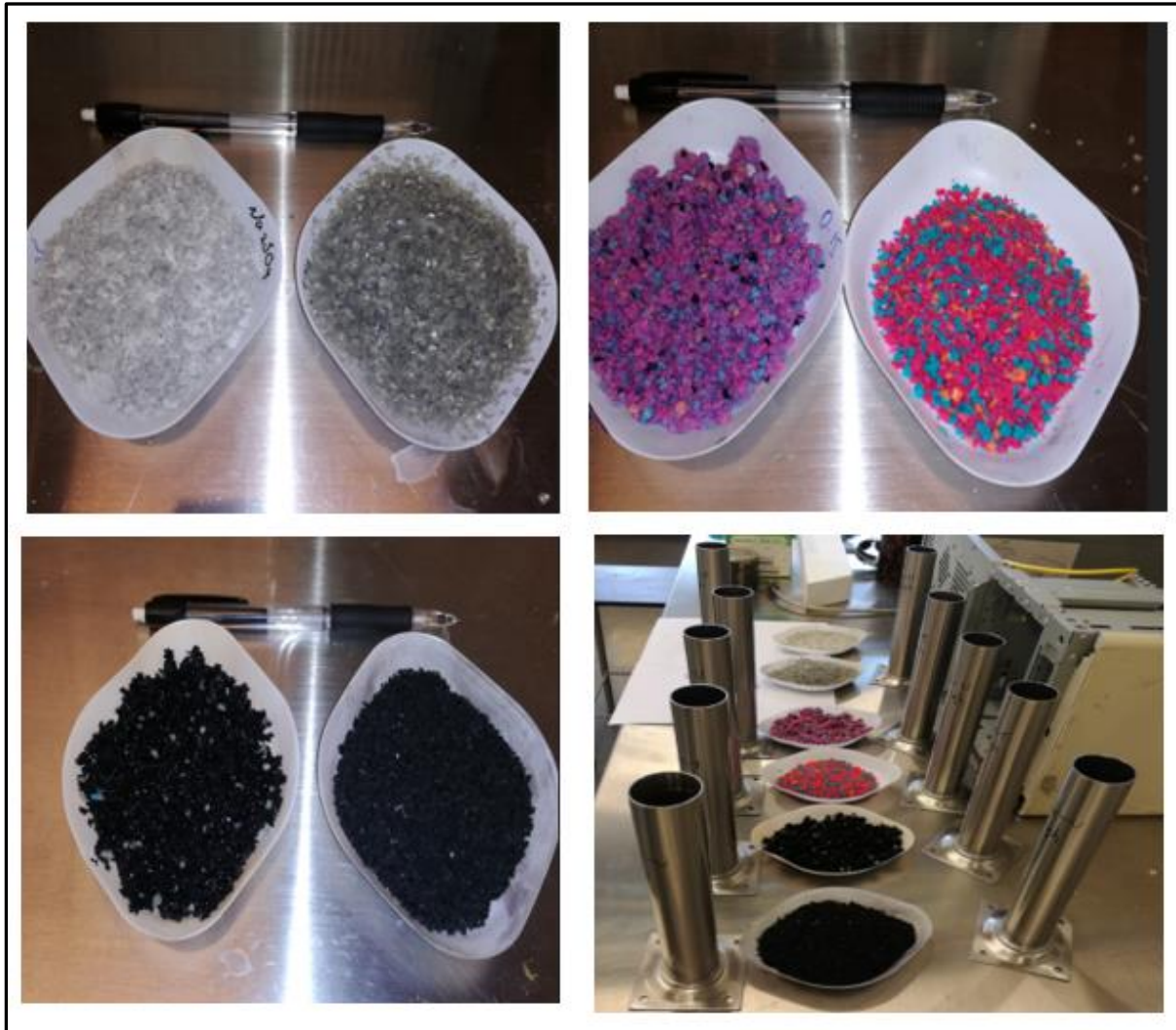
Figure 3-4: From top left to bottom right: Grey silicone (treated and untreated), red silicone (treated and untreated), tyre rubber (treated and untreated) & the collective batch of rubber specimens (Aarnes 2018)
