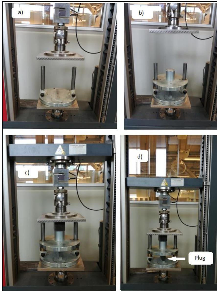
Figure 3-21: Modifications to repurpose the compressive apparatus, step by step. d) Shows the assembled test setup (Aarnes 2018)
