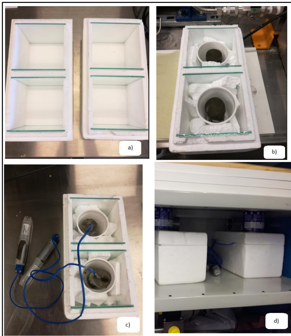
Figure 3-15: a) 4x 1.0-liter empty polystyrene compartments, b) cut polystyrene pieces to help isolate, c) temperature sensors installed in cement, d) packed and sealed boxes, stored in a cupboard (Aarnes 2018)
