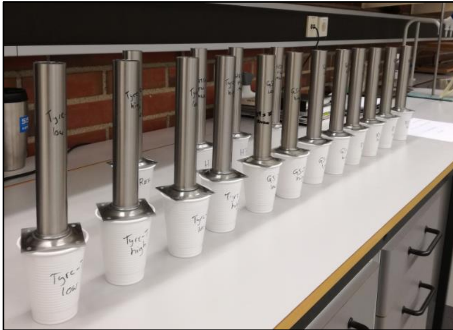
Figure 3-17: Cased cement, placed on top of plastic cups to measure leakage, if any, through or around the cement after heat treatment (Aarnes 2018)
