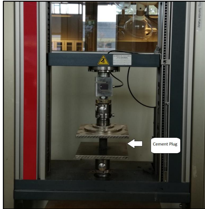
Figure 3-19: Zwick Z020 apparatus for destructive testing (Aarnes 2018)
