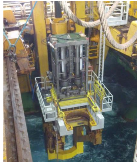
Figure 3. 4 Subsea Pump Module Placed in Launch System Prior to Docking to Riser [76]
