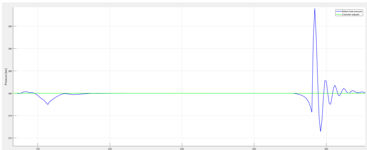
Figure 19 bottom hole pressure 20 second ramping
